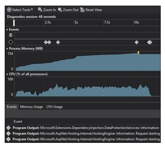
You can see the CPU and memory profiles, including the automatic Garbage Collection events that are used to free up memory (the marker just prior to memory use decreasing). You will be able to see breakpoint events and, if you have the enterprise version of VS, IntelliTrace events as well.
