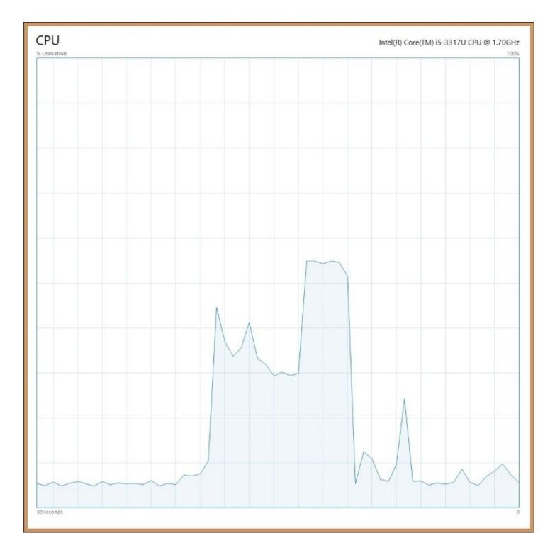
In the preceding graph, we can see that initially, when hashing in series, the CPU is running at about 25%, fully using one logical CPU. When hashing two passwords in parallel, it uses 50%, running on two logical processors. This doesn't translate into a twofold increase in speed due to the intrinsic overheads and the nature of **hyper-threading**.
