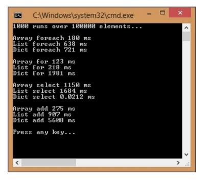
These results, shown in the preceding image, are informative, but you should be skeptical, as many things can skew the output, for example, the ordering of the tests. If the gap is small, then there is probably not much to choose between two variants, but you can clearly see the big differences.
