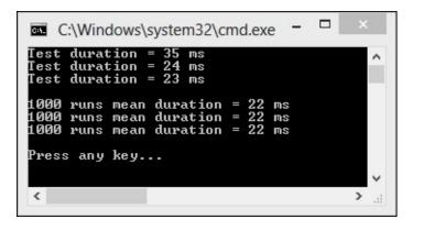
You can see that the three individual tests can give wildly different results and yet the averaged tests are identical.
