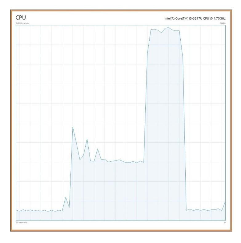
We can see that now the initial 25% usage jumps to almost full utilization and we are making use of most of the processor. This translates to just under a doubling of the performance as compared to hashing in sequence. There are still significant overheads involved, but, as the main operation is now so much quicker, the tradeoff is worth it.
