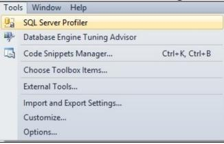
2. Load SQL Server Profiler and connect to the database that you are using. Name your trace and select the **Tuning** profile template.
