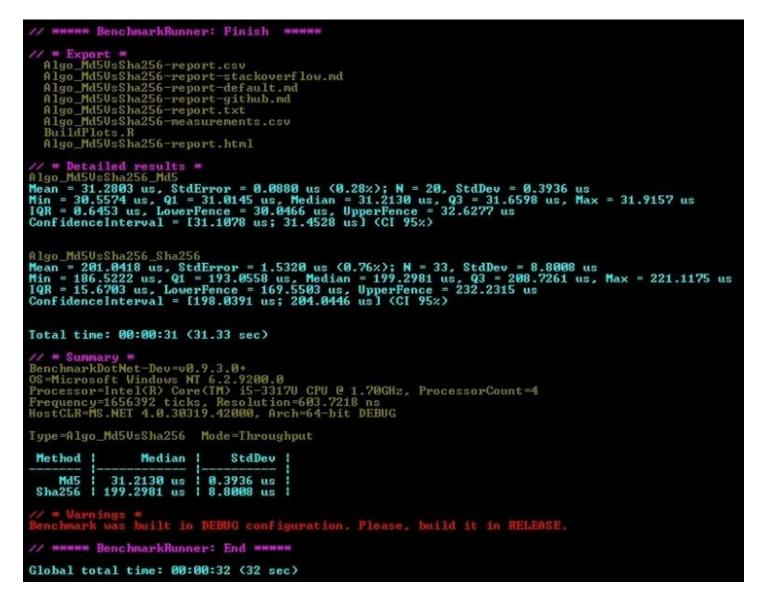
You can see in the last image that the results are different to our homemade benchmark. However, this uses the full .NET Framework, calculates median rather than mean for the average time, and runs in debug mode (which it helpfully warns us of) among other things.
