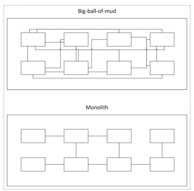
The large boxes represent the code running on each web server (the **Web Server N** boxes from the monolith example in the earlier diagram). From the outside, they look the same, but the difference is in the internal coupling of the code.
