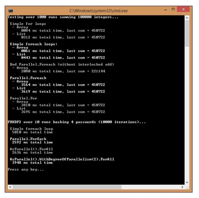
When calculating a sum, by accumulating 100,000 random integers between zero and ten, the quickest way is to use an array in a simple foreach loop. Using parallelization here makes the process much slower, and if used Naïvely, without locking, will give an incorrect result, which is much worse.
