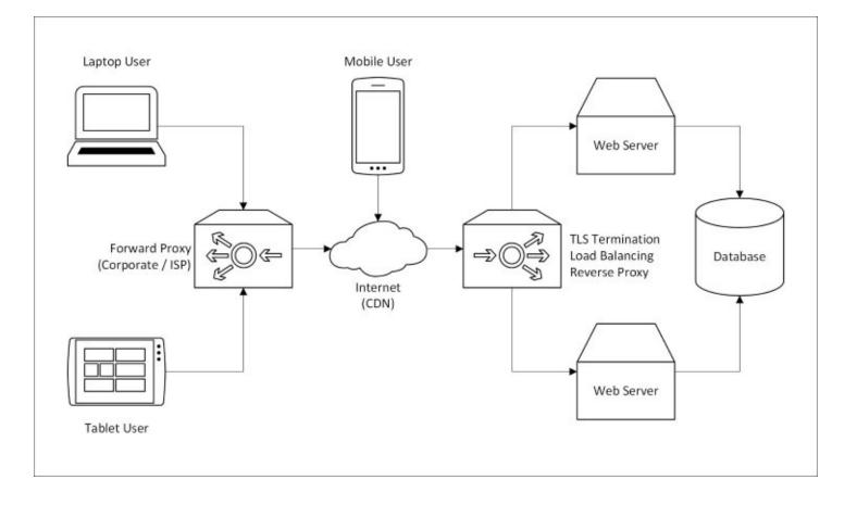
As seen in the preceding diagram, the laptop and tablet users are connecting through a caching forward proxy server (which may be on a corporate network or at an ISP). The mobile user is connecting directly over the internet. However, all users are going through a CDN before reaching your infrastructure.
