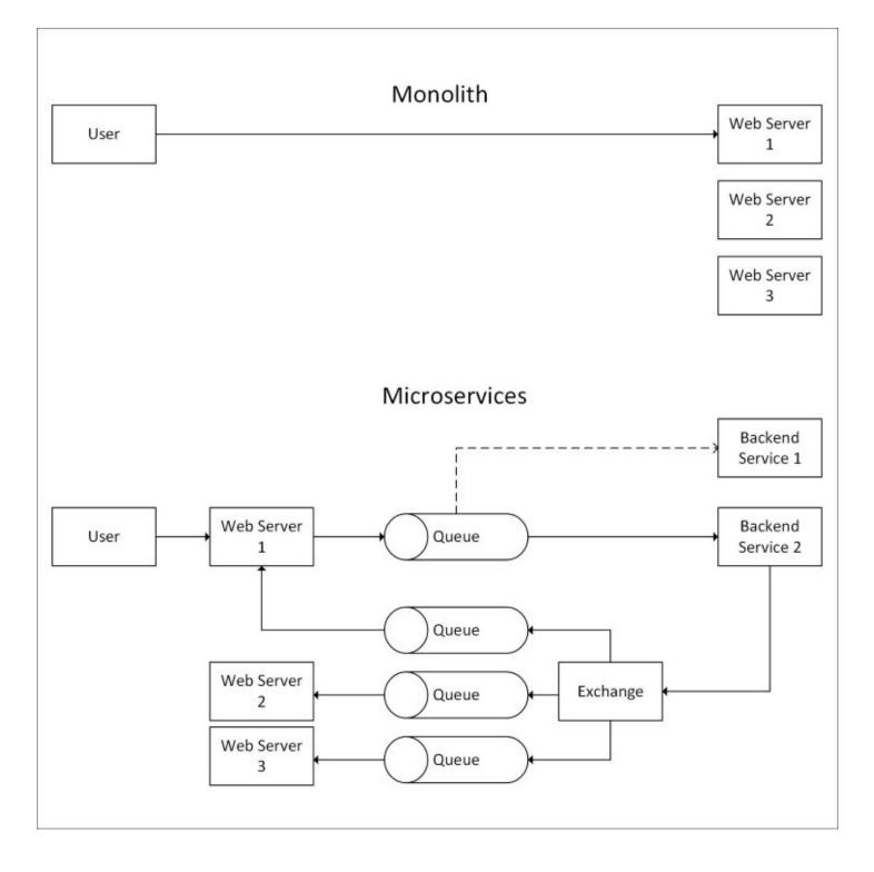
Here, the user makes a request to an application running on a web farm. We have omitted firewalls, load balancers, and databases for clarity, but multiple web servers are shown to illustrate that the same codebase runs on multiple machines.
