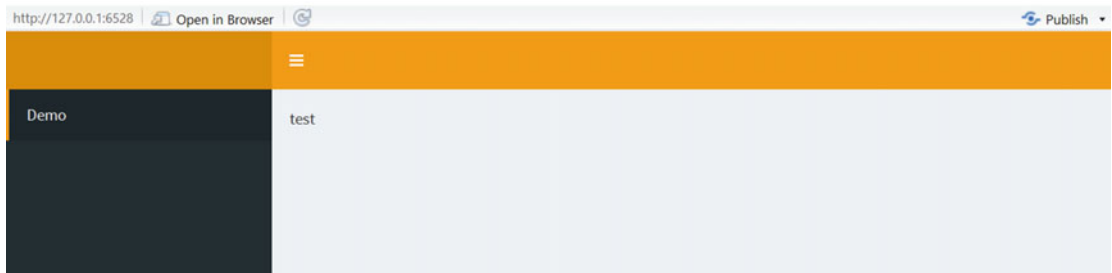
Figure 14-3. A dashboard with a menuItem() in the sidebar and a tabItem() in the body. Notice the matching First .
