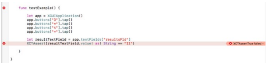
Figure 5-10. Failing test in Xcode
