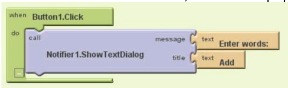
Figure 1-29: When the user clicks the button, the notifier displays a dialog box.
