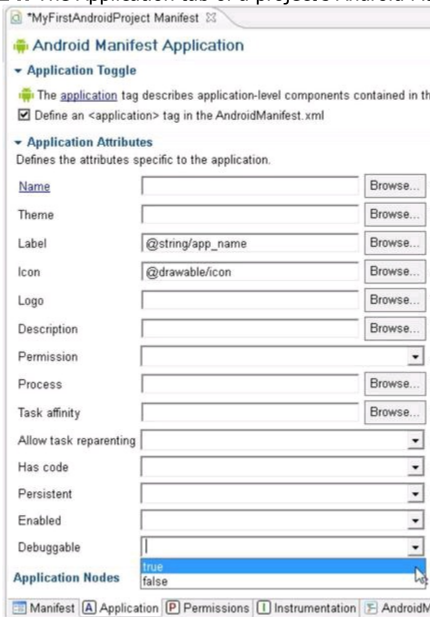
Figure 3-14: The Application tab of a project's Android Manifest.xml file.
