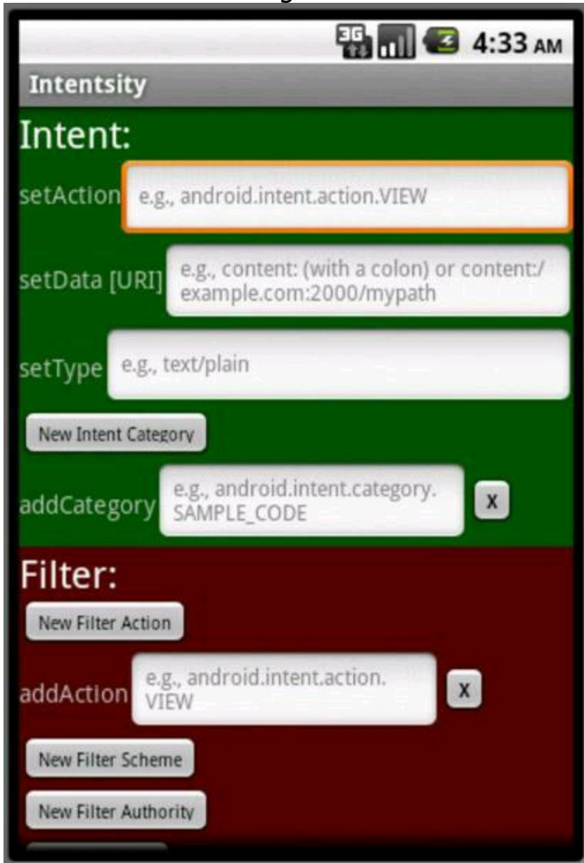
Figure 2-8: A screen for entering intent and intent filter strings.
