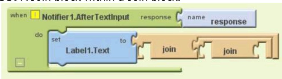
Figure 1-33: A Join block within a Join block.
