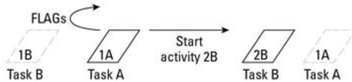
Figure 2-19: The effect of adding FLAG_ACTIVITY_REORDER_TO_FRONT. Without FLAG_ACTIVITY_REORDER_TO_FRONT:
