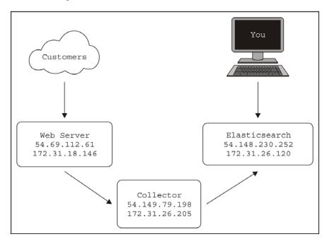
For this example, I'll start three servers in Amazon's **Elastic Compute Cluster** (**EC2**), as shown in this diagram:
