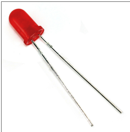
Figure 4-11: A lone LED, ready to be put to work.
