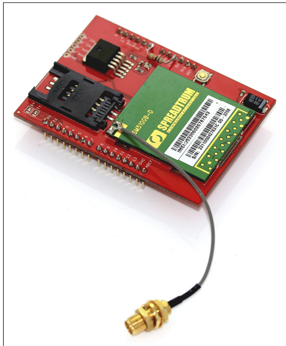
Figure 13-9: The Cellular Shield ready to connect people.
