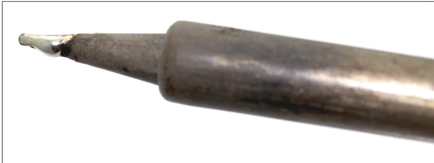
Figure 10-16: Tinning the tip helps to preserve your iron and makes soldering easier.
