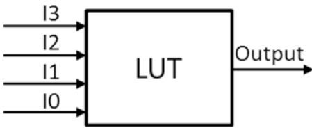
Figure 1-3. Four inputs, one output Boolean function
