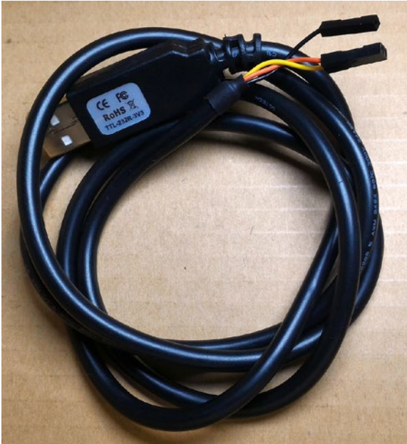
Figure 13-3. USB to UART cable—TTL-232R-3V3/TTL-232R-RPI
