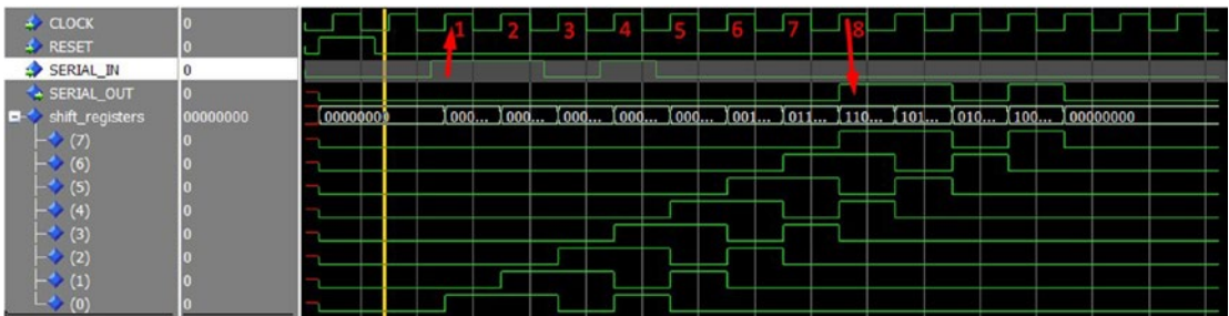
Figure 10-6. Simulation result for 8-bit SISO Shift register
