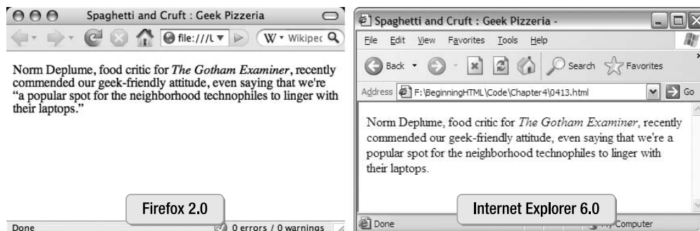
Figure 4-13. A view of the same markup from two different browsers: Firefox draws the punctuation, but Internet Explorer doesn't.
