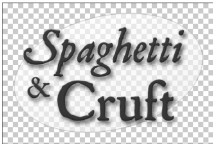
Figure 5-4. A 24-bit PNG with a transparent alpha channel. The checkerboard background shows through the translucent parts of the image.
