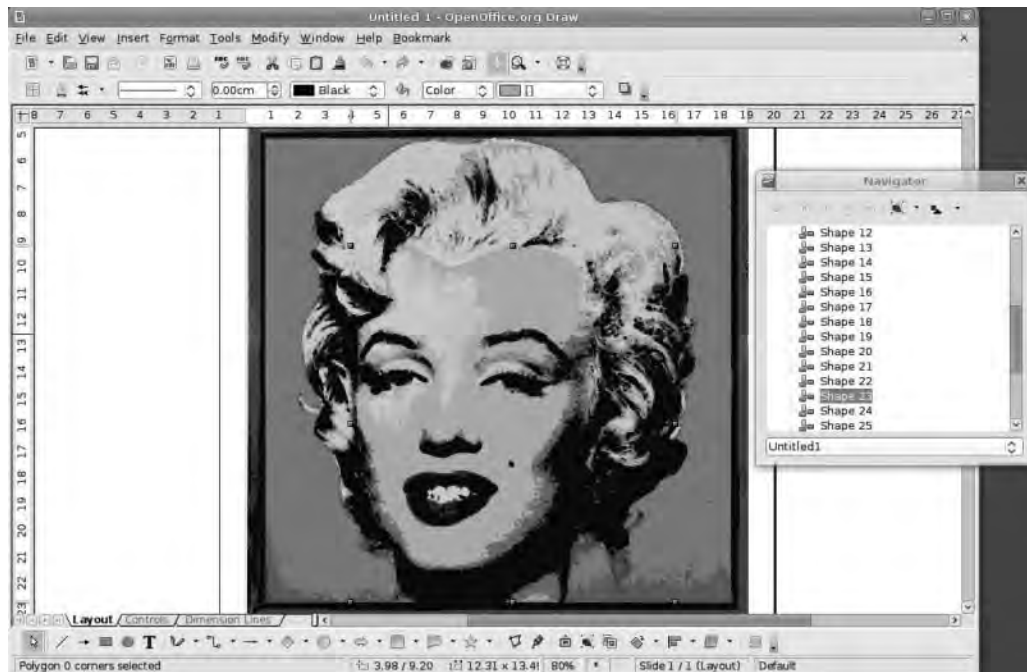
Figure 6-41. Warhol's Monroe screen print is the ideal vectorization project. By selecting 32 colors in the dialog box, you end up with 32 colored regions that you can easily edit.
