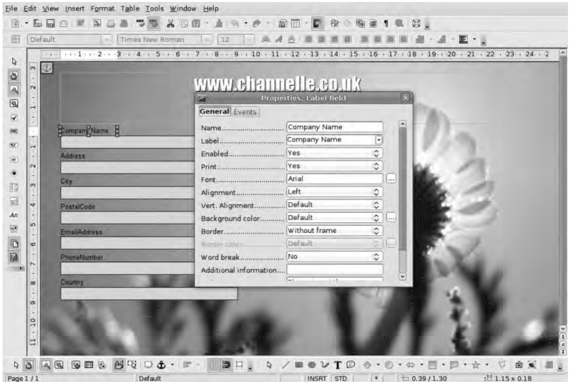
Figure 7-18. Changing the label on a form will have no impact on the database information itself, so you can tailor the label to the audience.
