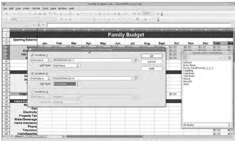
Figure 4-32. The modulo function can be used to format the look of odd or even rows to create a zebra effect on the spreadsheet.
