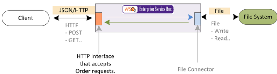
Figure 7-5. Using File Connector to execute various file system operations from a mediation flow
