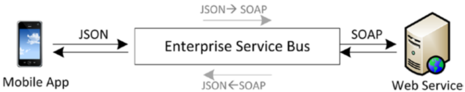
Figure 1-1. An ESB can be configured to convert messages between the formats recognized by the mobile app (JSON) and the web service (SOAP) it wants to talk to. This is a simple example of enterprise integration.
