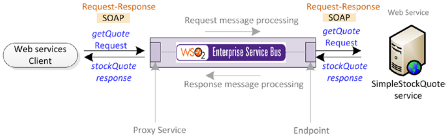
Figure 4-2. In synchronous messaging when the web service client sends a request, it waits and expects a response message. WSO2 ESB supports synchronous messaging between the client and ESB, and also between ESB and the backend service.
