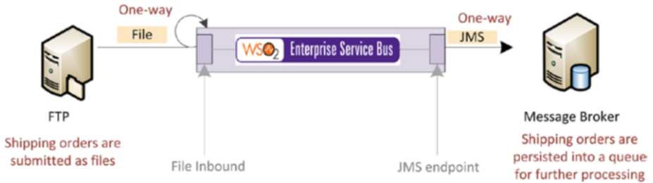
Figure 4-15. Fetching the shipping orders stored in the FTP by using a file inbound endpoint, processing them, and then adding them to message queue via JMS protocol
