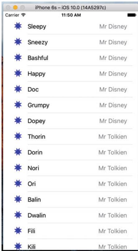
Figure 8-12. The style value1 places the text label on the left side in black letters and the detail text right-justified on the right side
