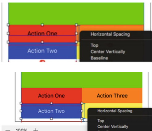
Figure 5-23. Attach each row of buttons together at the center of the view; this, by default, sets the width of each button to be half the width of the view
