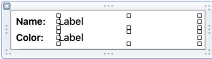
Figure 8-25. The table view cell's content view with the left label names changed and set to Headline style, which is bold, and with the right labels slightly moved and resized
