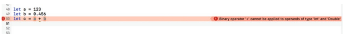
Figure A-5. Swift does not allow you to combine variables of different types
