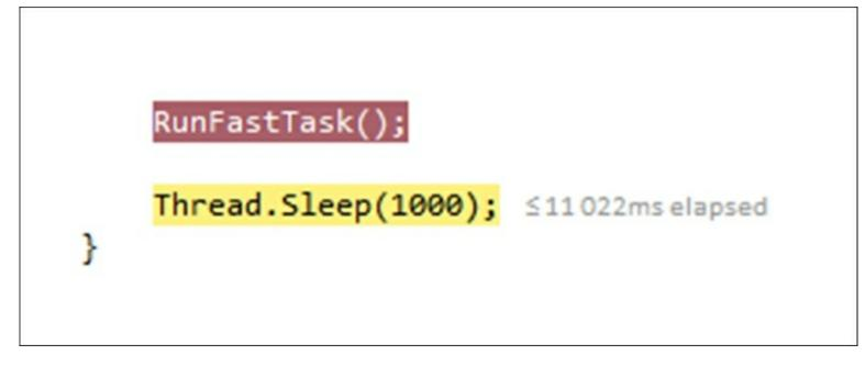
6. Stepping in to the RunFastTask() method, you can place further breakpoints and step over them one by one to find the method that is causing the longest delay. As you can see, PerfTips allow developers to quickly and easily identify bottlenecks in code:
