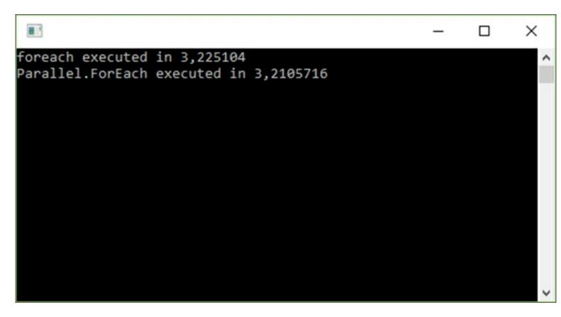
7. Let's use a different example now. We will create a process-intensive task and measure the performance gain that the Parallel.ForEach loop will give us. Create two methods called CreateWriteFilesForEach() and CreateWriteFilesParallelForEach(), which both take the List<string> collection as the parameter:
