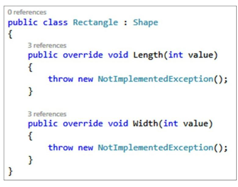
13. To add implementation to our Rectangle class, create two properties for the Length() and Width() methods and set these properties equal to the value of the supplied parameter value:
