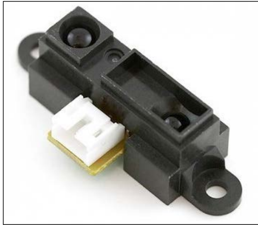
The infrared Sharp GP2Y0A-family sensor
