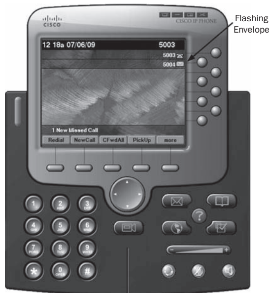
FIGURE 8.1 Flashing envelope MWI
