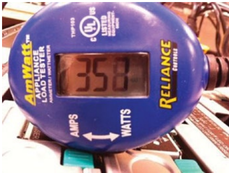
Figure 5-3. Power draw of a cloud platform baseboard running the Intel PTU stress test
