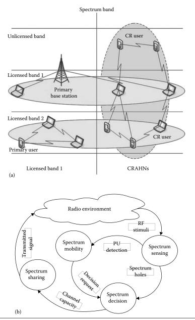
Figure 1.4 The CRAHN architecture (a) and the CR cycle (b).
