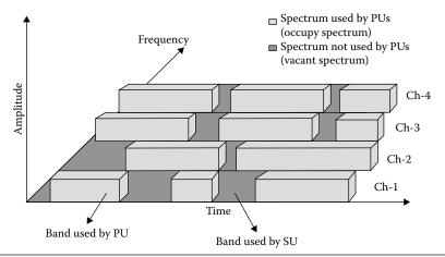
Figure 6.2 CRN concepts: Spectrum holes.
