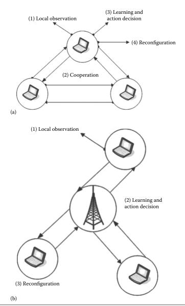
Figure 1.3 Comparison of CR capabilities between infrastructure-based CR networks (a) and CRAHNs (b).
