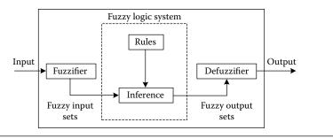
Figure 2.11 The structure of an FLS.
