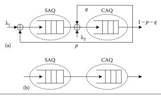
Figure 2.6 Queuing models for SCDQMAC (a) and MCDQMAC (b).
