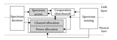
Figure 1.11 Spectrum sharing structure for CRNs.
