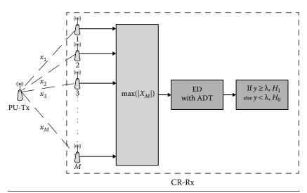
Figure 6.11 Proposed model: ED\_MA\_ADT. Tx, Transmitter.
