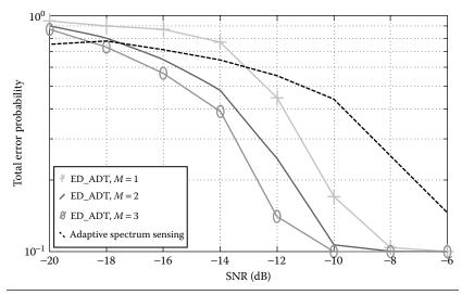
**Figure 6.14** Probability of error versus SNR at  $P_{\rm f} = 0.1$  with N = 1000, number of antennas M = 1, 2, 3, QPSK modulation scheme, and Rayleigh fading channel.
