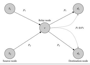
Figure 8.2 A sample example of multipath NC.
