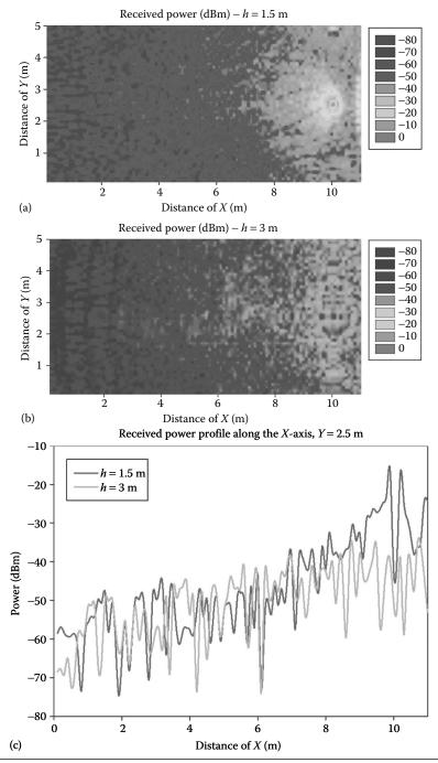
**Figure 7.12** Estimations of received power levels considering Bluetooth transceivers. The impact of multipath propagation can be seen in the power delay profile estimations, which derive in an overall delay spread of 76.4549 ns.
