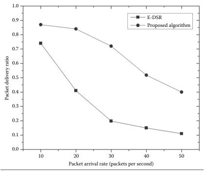
**Figure 11.2** Packet delivery ratio with different message generation rates under different routing protocols.
