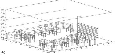
**Figure 7.6** Scenario employed in order to analyze topomorphological impact on different wireless systems: (a) Image of the test scenario; (b) implemented simulation model.
