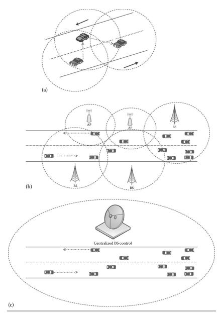
**Figure 14.3** Three main scenarios of architectures' deployment for CRNs. (a) Vehicle-to-vehicle communications; (b) multi local heterogeneous wireless communications; (c) centralized wireless communications.
