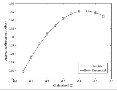
**Figure 12.8** Aggregated throughputs versus CI threshold  $\xi$ .
