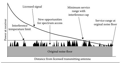
Figure 5.9 Interference temperature model.
