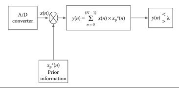
Figure 6.4 Matched filter detector. A/D, Analog to digital converter.
