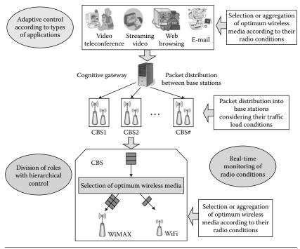
Figure 2.16 The frame of adaptive route control.
