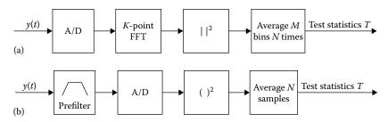
**Figure 5.6** Digital implementation of energy-based detection (a) with periodogram: FFT magnitude squared and averaged (b) with analog prefilter and square-law device. (Data from D. Cabric, et al., "Spectrum Sensing Measurements of Pilot, Energy, and Collaborative Detection," *Proceedings of the IEEE Military Communication Conference*, October 2006, pp. 1–7.)
