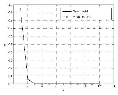
**Figure 4.4** Distribution of the number of packets in the system in a scenario with p = .0002.
