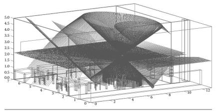
Figure 7.2 Typical scenario of an office with the rays launched from the transmitter.
