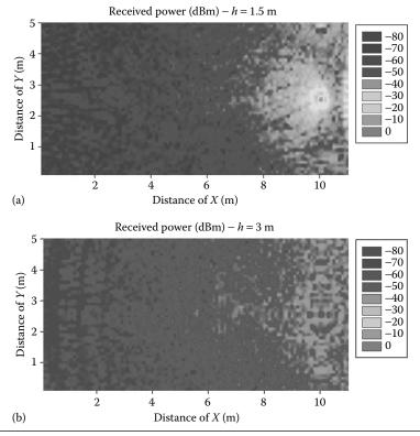
**Figure 7.13** Estimations of received power levels considering Bluetooth v4.0 transceivers. The impact of multipath propagation can be seen in the power delay profile estimations, which derive in an overall delay spread of 84.0497 ns.
