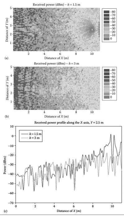
**Figure 7.11** Estimations of received power levels in ZigBee systems in the case of 2.4 GHz band. The impact of multipath propagation can be seen in the power delay profile estimations, which derive in an overall delay spread of 32.8761 ns.
