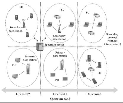
Figure 2.3 Network architecture of dynamic spectrum sharing.
