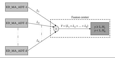
Figure 6.17 CSS technique based on ED\_MA\_ADT in CRNs.
