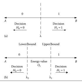
Figure 6.9 (a) Conventional detection method with single-threshold scheme; (b) hierarchical spectrum sensing method with double-threshold scheme.
