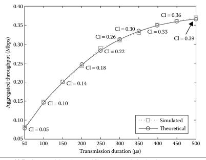
Figure 12.7 Aggregated throughputs and CI versus transmission durations.
