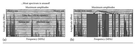
**Figure 1.1** Spectrum is wasted. Opportunistic spectrum access can provide improvements in spectrum utilization. (a) Spectrum usage by traditional spectrum management, (b) spectrum usage by utilizing spectrum holes.
