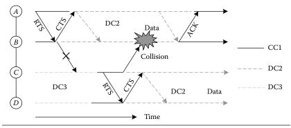
Figure 2.18 The multichannel hidden terminal problem.
