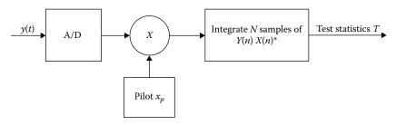
**Figure 5.5** Pilot signal and MF-based detection. (Data from D. Cabric, et al., "Implementation Issues in Spectrum Sensing for Cognitive Radios," *Asilomar Conference on Signals, Systems and Computers*, Pacific Grove, CA, June 2004, pp. 772–776.)
