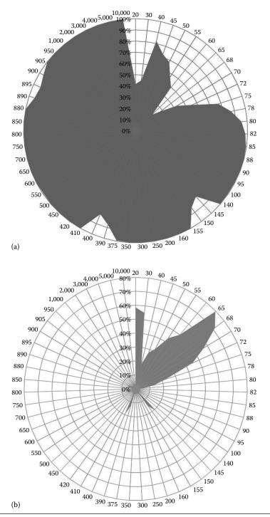
Figure 7.17 Messages received (a) and lost (b) for different transmission periods.
