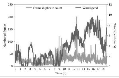
Figure 13.5 Evolution of duplicate frame count versus wind speed over time.
