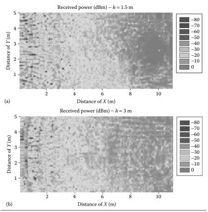
**Figure 7.10** Estimations of received power levels in ZigBee systems in the case of 868 MHz band. The impact of multipath propagation can be seen in the power delay profile estimations, which derive in an overall delay spread of 32.8761 ns.
