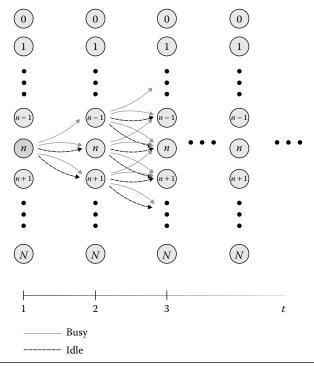
Figure 4.5 Full trellis diagram associated with the transition diagram in Figure 4.2.
