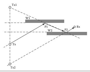
Figure 7.1 Illustration of the image method.
