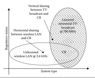
**Figure 5.3** Spectrum sharing by SUs with different types of systems depending on regulatory status of incumbent radio systems: vertical and horizontal sharing of spectrum.
