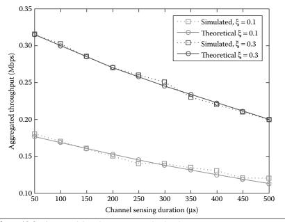
Figure 12.9 Aggregated throughputs versus sensing duration.
