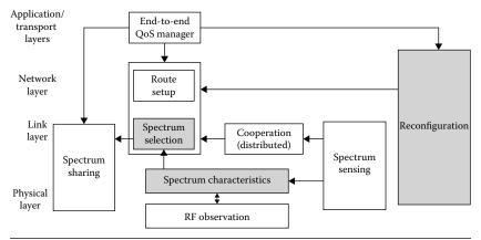
Figure 1.10 Spectrum decision structure for CRAHNs.
