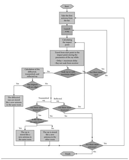
Figure 7.3 Functional diagram of the 3D ray launching algorithm.
