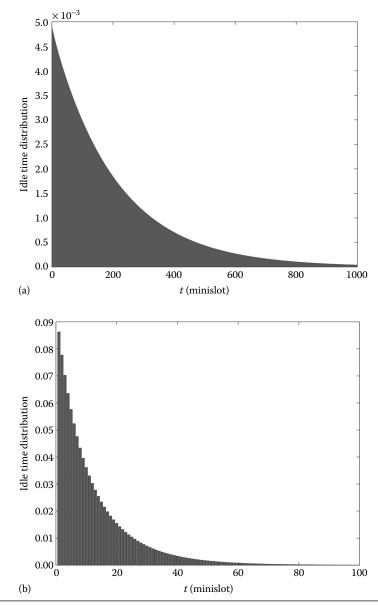
**Figure 4.7** Idle time distributions corresponding to various values of p: (a) .0002; (b) .003; (c) .007; (d) .01. In all cases, N = 12 and L = 10.
