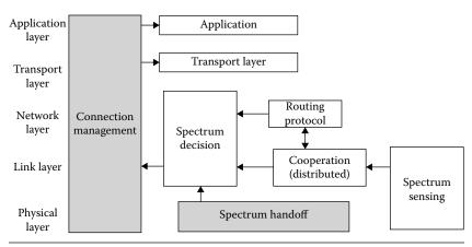
Figure 1.14 Spectrum mobility structure for CRAHNs.
