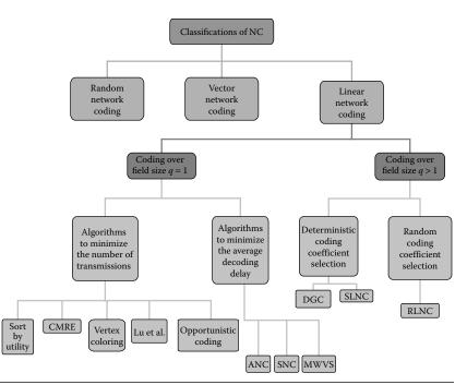
**Figure 8.4** Classification of NC. CMRE, cache-based multicast retransmission encoding; DGC, dynamic general-coding; MWVS, maximum weight vertex search; RLNC, random linear network coding; SLNC, sparse linear network coding.
