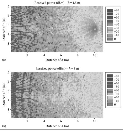
**Figure 7.8** Estimations of received power levels in WLAN systems. The impact of multipath propagation can be seen in the power delay profile estimations, which derive in an overall delay spread of 74.25047 ns.
