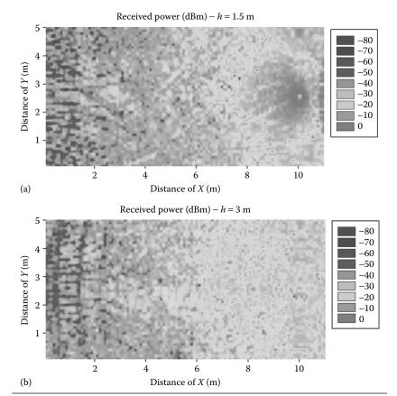
**Figure 7.7** Estimations of received power levels in 3G UMTS systems. The impact of multipath propagation can be seen in the power delay profile estimations, which derive in an overall delay spread of 74.3 ns.: (a) Estimation of received power for h = 1.5 m; (b) Estimation of received power for h = 3 m; (c) received power profile for both heights; (d) Power Delay Profile estimation.
