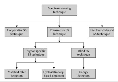
Figure 6.3 CRN spectrum sensing techniques. SS, spectrum sensing.
