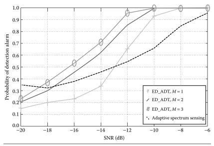
**Figure 6.13** Probability of detection versus SNR at  $P_i = 0.1$  with N = 1000, number of antennas M = 1, 2, 3, QPSK modulation scheme, and Rayleigh fading channel.
