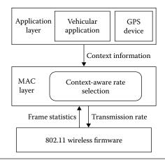
**Figure 14.2** The system architecture of the proposed CARS. GPS, global positioning system; MAC, media access control layer. (Data from Shankar, P. et al., CARS: Context-aware rate selection for vehicular networks, *IEEE International Conference on Network Protocols*, pp. 1–12, Orlando, FL, October 19–22, 2008.)
