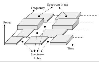
Figure 1.2 Spectrum holes concept.
