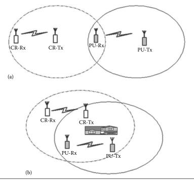
Figure 5.8 Hidden PU problem because of path loss (a) and shadowing/blocking (b).
