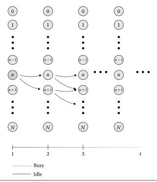
**Figure 4.6** Reduced trellis diagram, with only branches associated with idle minislots, derived from the full trellis diagram in Figure 4.5.
