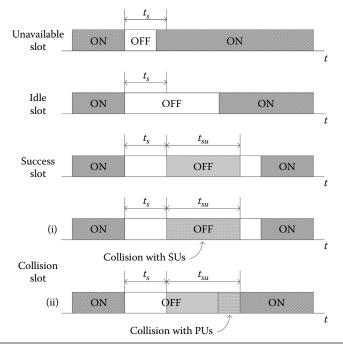
Figure 12.5 Virtual slot model to represent various OFF slots.
