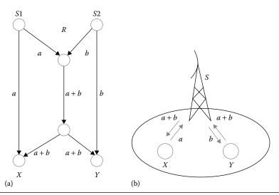
Figure 8.1 NC examples: (a) Multicast with two sources and two receivers; (b) wireless pointto-point communication.
