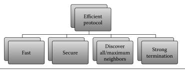
Figure 3.2 Features of an efficient ND protocol.
