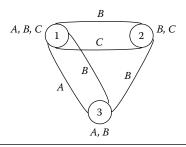
**Figure 2.10** A Network color graph (NCG) representation of channel availability and interference constraints. (H. Zheng and C. Peng, "Collaboration and fairness in opportunistic spectrum access," *Proceedings of the IEEE International Conference on Communications*, vol. 5, pp. 3132–3136, May 2005.)
