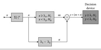
Figure 6.12 Internal architecture of ED with ADT scheme.
