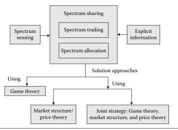
Figure 2.8 Solution for spectrum sharing in CRNs.
