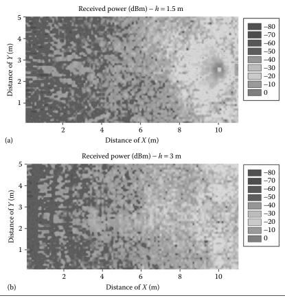
**Figure 7.9** Estimations of received power levels in WLAN systems in the case of 5 GHz band. The impact of multipath propagation can be seen in the power delay profile estimations, which derive in an overall delay spread of 74.25047 ns.
