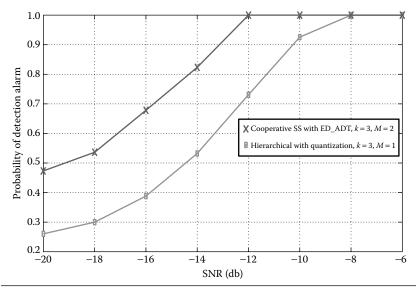
**Figure 6.18** Probability of detection versus SNR at  $P_f = 0.1$  with N = 1000, M = 2, total number of cooperative CR users k = 3, QPSK modulation scheme, and Rayleigh fading channel.
