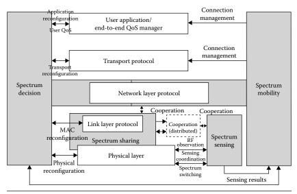
Figure 1.5 Spectrum management framework for CRNs.
