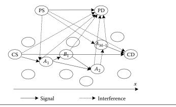
**Figure 2.13** The primary transmission coexists with the multihop cognitive transmission.
