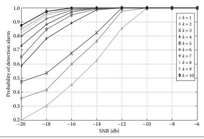
**Figure 6.19** Probability of detection versus SNR at  $P_i = 0.1$  with N = 1000, M = 2, k = 1, 2, ..., 10, QPSK modulation scheme, and Rayleigh fading channel.
