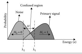
Figure 6.7 Energy distribution of PU signal and noise.
