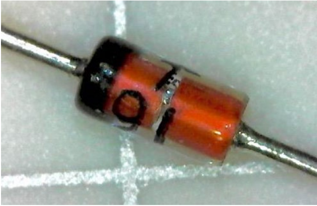
Figure 6-11. 1N914 diode to be tested
