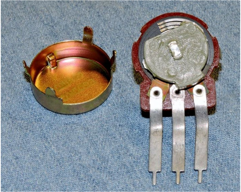
Figure 7-2. The revealed innards of a PCB potentiometer
