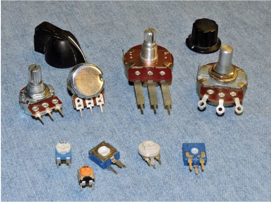
Figure 7-1. A small collection of different potentiometers
