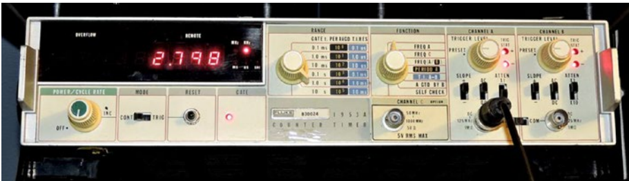
Figure 5-3. An old Fluke 1953A frequency counter used to determine the 3.3V formula for C_1 by measuring frequency
