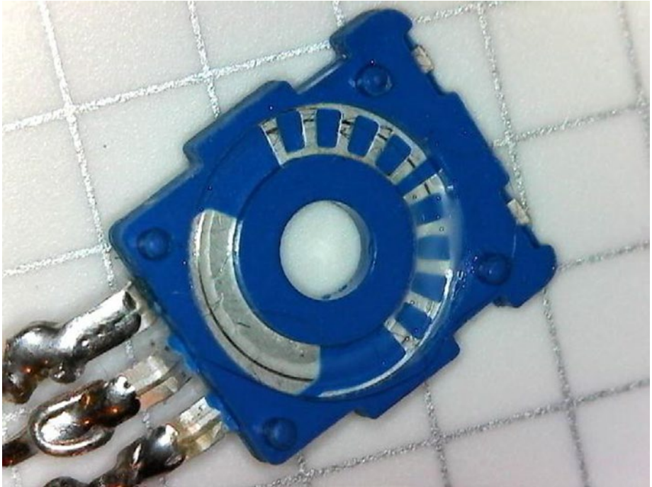
Figure 8-2. Contact side of the rotary encoder
