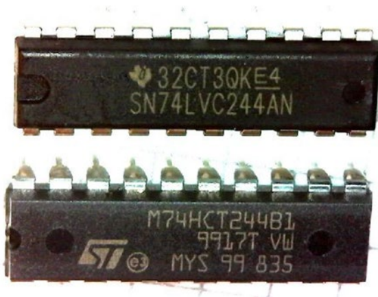
Figure 2-1. Two useful level interfacing chips
