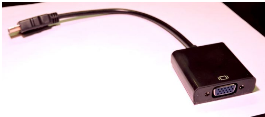
Figure 3-1. HDMI to VGA adapter
