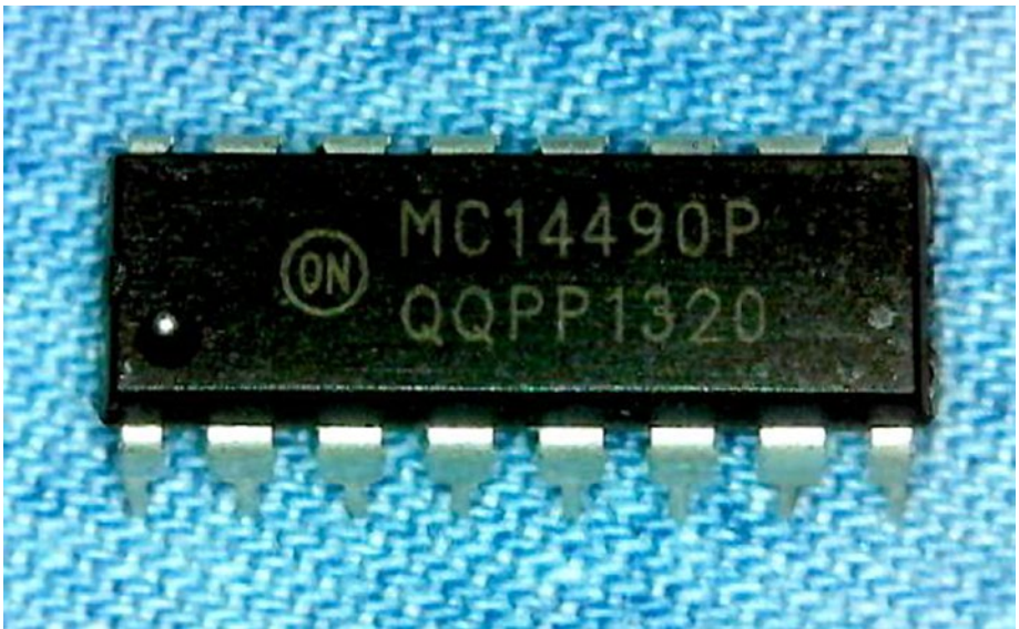
Figure 5-1. The MC14490 dual inline package (DIP) chip
