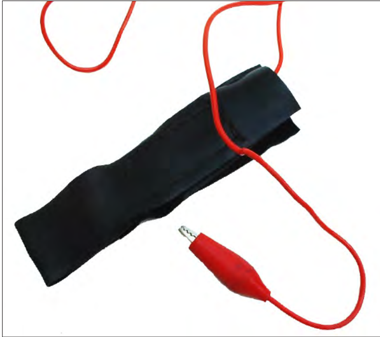
Figure 9-6: An anti-static wrist strap reduces or eliminates the risk of electrostatic discharge.
