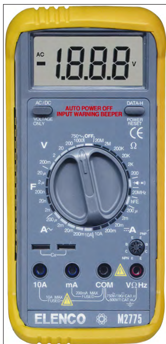
Figure 9-2: Multimeters measure voltages, resistance, and current.
