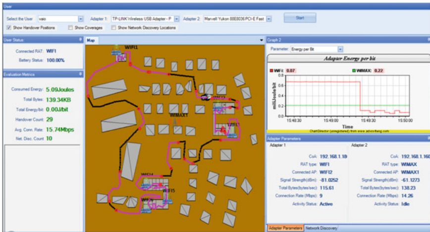
Fig. 8.17 Trace of handovers using energy efficient vertical handover algorithm [5]
