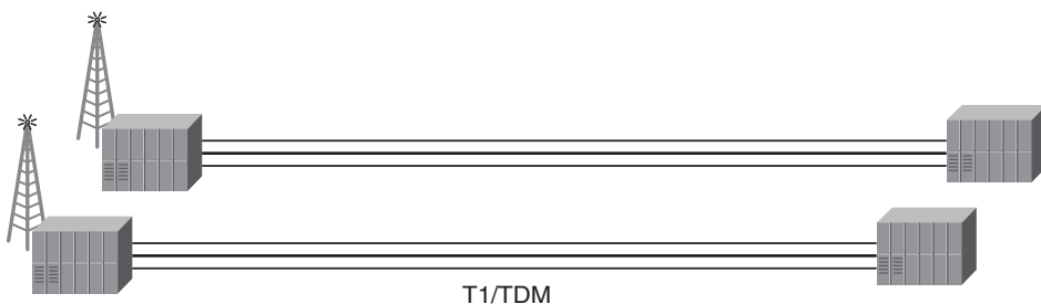
Figure 8-10 Load-Shared TDM Circuits
