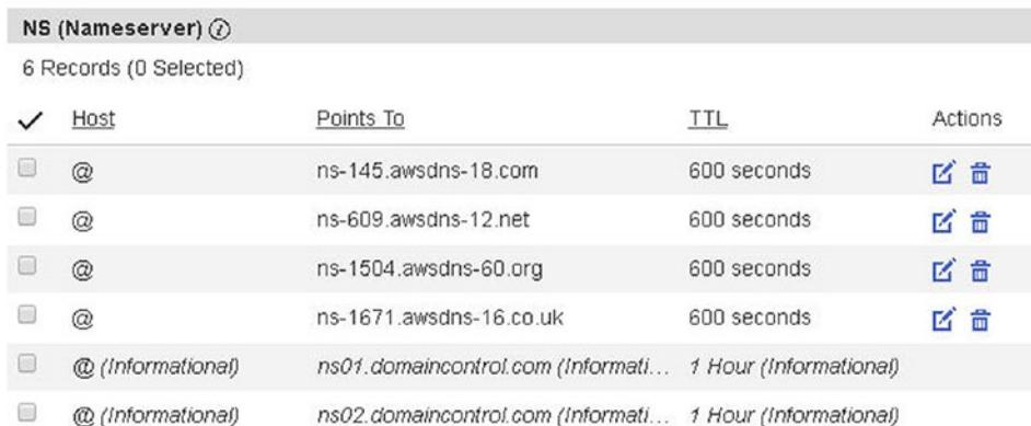
Figure 16-25. Adding name servers for Route 53 to DNS record
