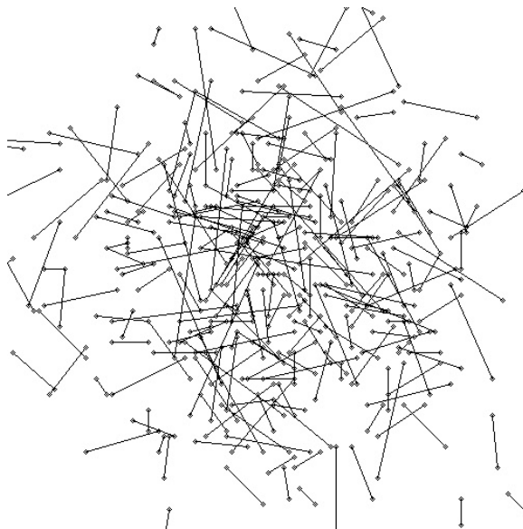
Figure 16-27. A visualization of pixel-to-pixel tests that collectively comprise a single BRIEF descriptor; each line connects a pair of pixels that are compared by the test
