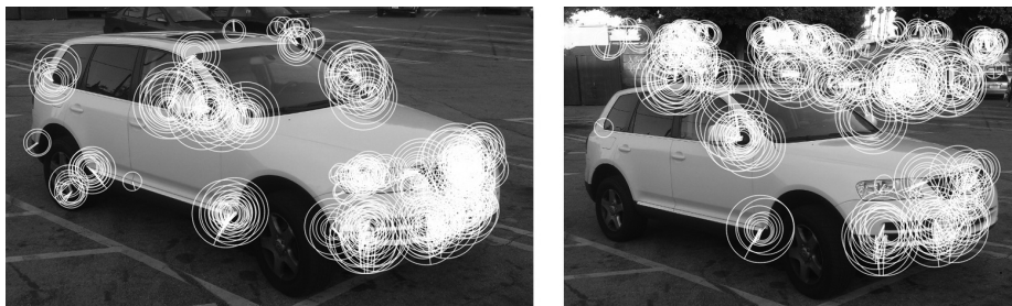
Figure 16-31. Two images of the same vehicle each produce 500 ORB features. An interesting characteristic of ORB is visible here, namely that if a corner is large in the image, many ORB features of differing sizes will be found on that same corner
