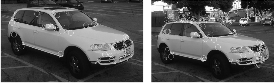
Figure 16-25. Star features computed for the same vehicle from two slightly different orientations. At default parameters, 137 are found on the left image and 336 are found on the right. In both cases, the number on the automobile is about the same, with the additional features on the background accounting for the greater number in the second image. The found features on the vehicle are few compared to other methods, but you can easily see correspondences, suggesting the features are very stable
