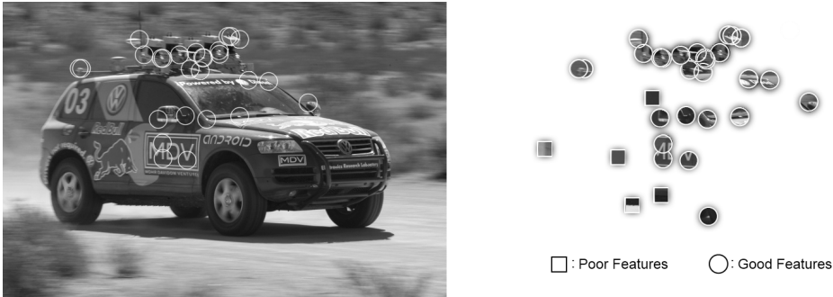
Figure 16-1. The points marked with circles here are good points to track, whereas those marked with boxes—even the ones that are sharply defined edges—are poor choices
