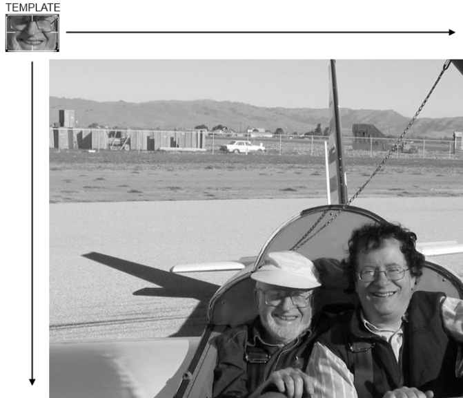
Figure 13-9. cv::matchTemplate() sweeps a template image patch across another image looking for matches
