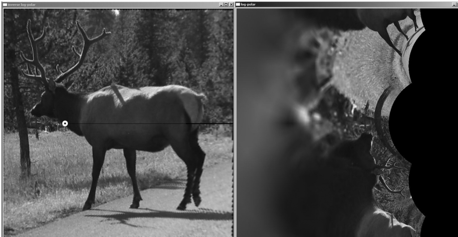
Figure 11-7. Log-polar example on an elk with transform centered at the white circle on the left; the output is on the right
