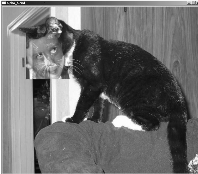
Figure 5-1. The face of a child, alpha-blended onto the face of a cat
