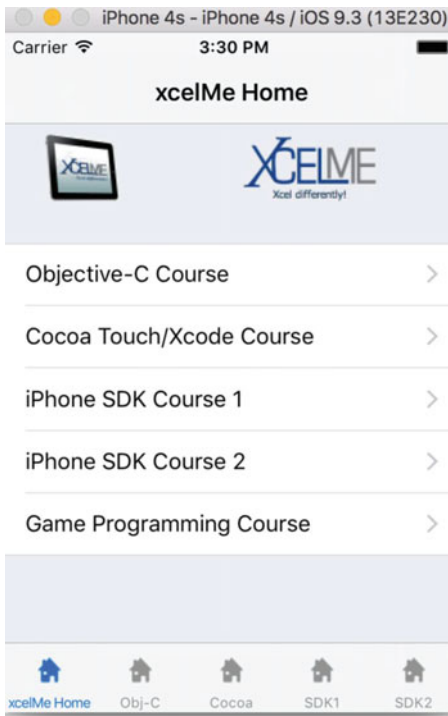
Figure 1-5. This sample iPhone app contains a table object to organize a list of courses. Actions such as “rotate left” or “user did select row 3” can be applied to this view object
