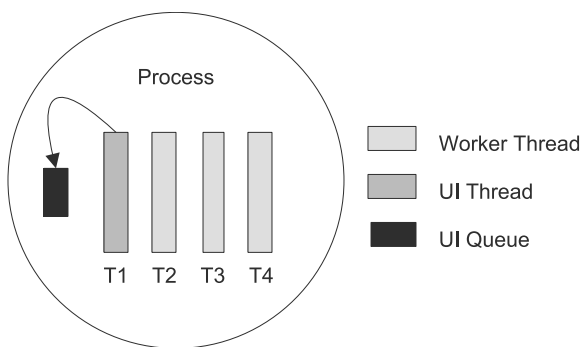
Figure 2-8. UI thread processing messages stored in a UI queue
