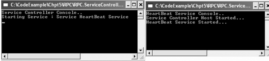
Figure 5-9. Console output of service controller and heartbeat service
