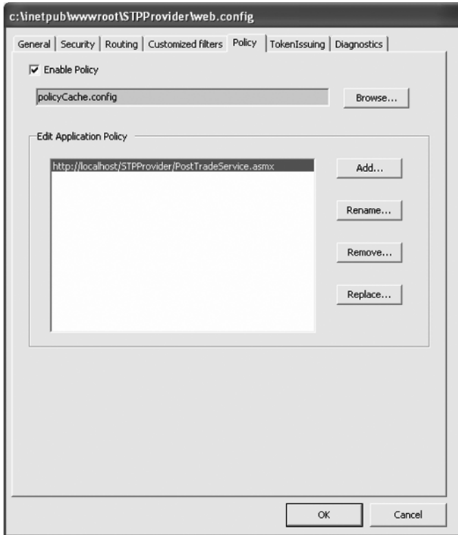
Figure 7-33. WSE configuration showing how to configure Web service policies
