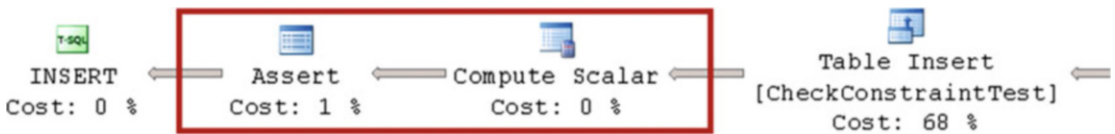
Figure 8-10. Part of the execution plan: insert with check constraint
