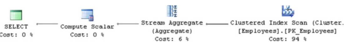
Figure 26-6. Parameter sniffing: OPTIMIZE FOR UNKNOWN hint
