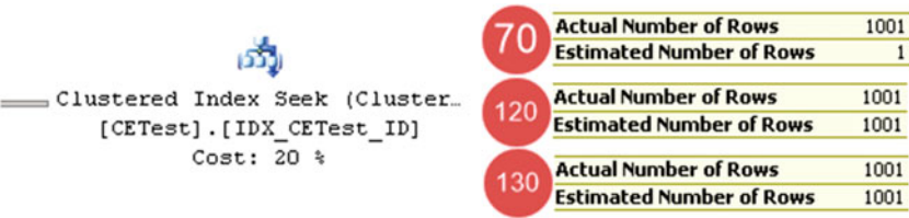
Figure 3-20. Cardinality estimations for indexes with ever-increasing keys
