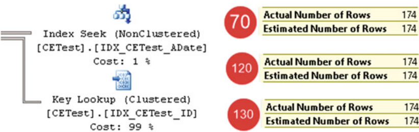
Figure 3-13. Up-to-date statistics: Cardinality estimations for a value that is a key in the histogram step
