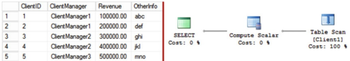
Figure 5-14. Row-level security: Data and execution plan without RLS applied
