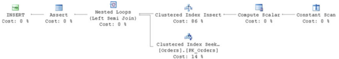
Figure 8-3. Inserting a row into the referencing table with a foreign key constraint defined
