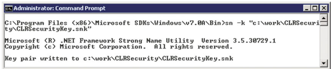
Figure 14-2. Generating key pair file with sn.exe
