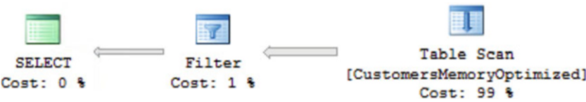
Figure 35-18. Composite hash index: Execution plans where query use the leftmost index column only (SQL Server 2016)
