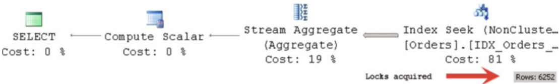
Figure 19-18. Execution plan for query with nonclustered index
