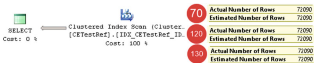
Figure 3-21. Cardinality estimations with join elimination
