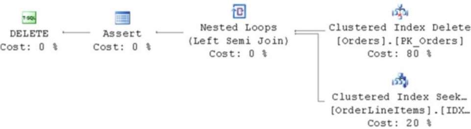
Figure 8-4. Deleting a row from the referenced table (no cascade actions)
