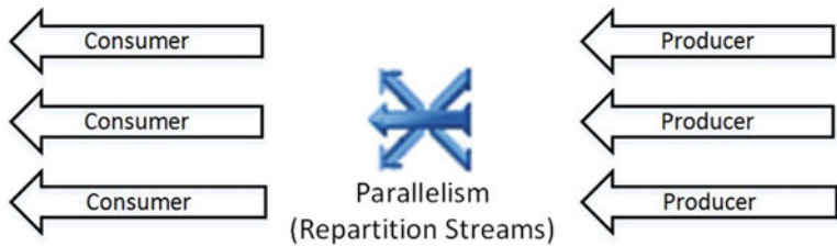
Figure 25-17. Parallelism: Repartition streams mode
