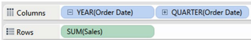
Figure 3-1. Dimension “Order Date” placed on columns shelf and the measure “Sales” placed on rows shelf
