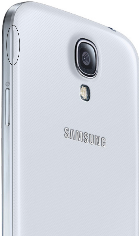
Figure 2-2: Open the cover from the slot at the top of your phone.
