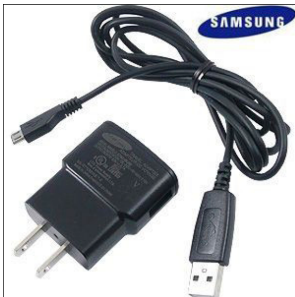
Figure 2-5: The transformer and USB cable for charging your phone.
