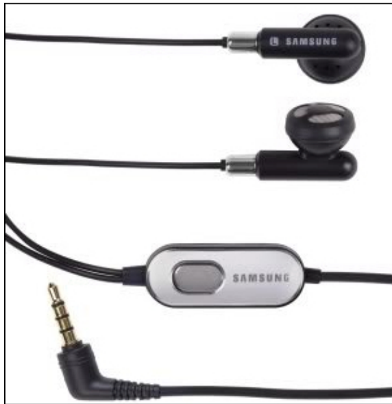
Figure 12-1: A typical wired headset with ear buds and a 3.5mm plug.
