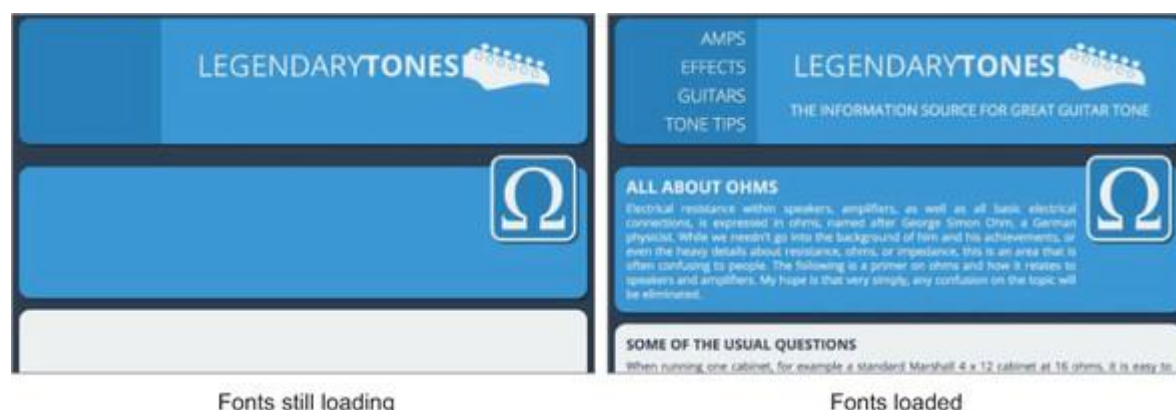
Figure 7.12. As a page loads embedded fonts, the text is initially invisible (left) until the fonts fully load, at which point the text styled in those font faces appears.
