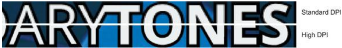
Figure 5.11. An enlarged visual representation of graphics on standard displays versus high DPI displays
