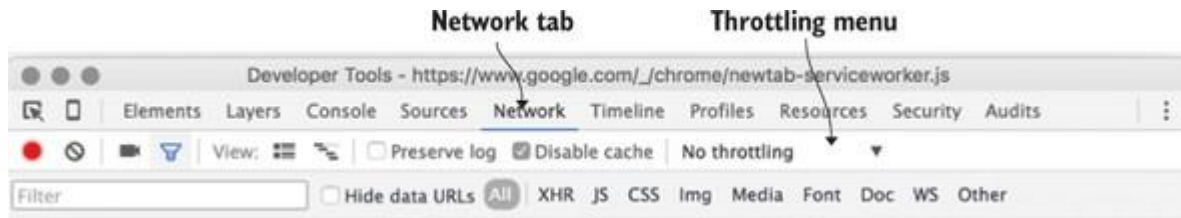
Figure 1.6. The location of the Network tab in the Google Chrome Developer Tools window. You can simulate internet connection speeds by using the throttling menu.
