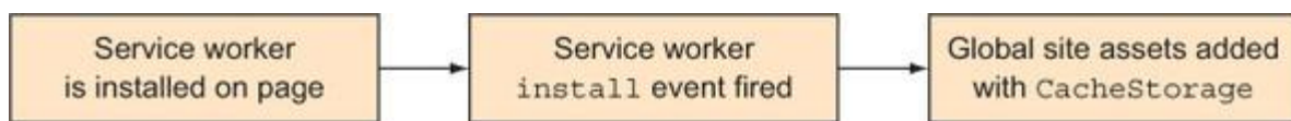
Figure 9.4. The behavior that you want to occur when the service worker's install event is fired
