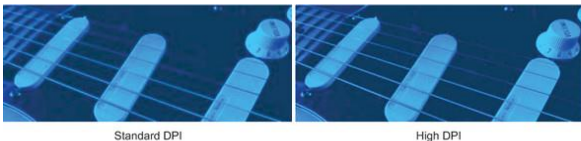
Figure 5.12. A comparison of two versions of a background image on two display types. On the left, a background image intended for use on standard displays appears on a high DPI display. On the right, the proper resolution image is used for the high DPI display, creating a better visual experience.
