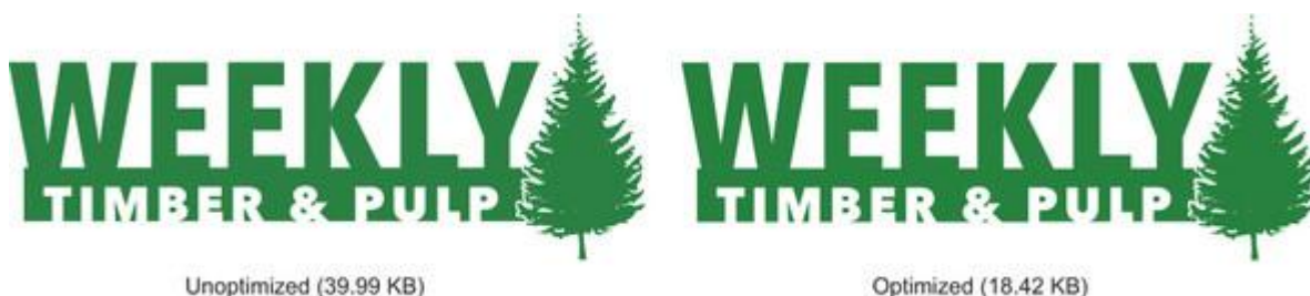
Figure 6.11. The Weekly Timber logo before (left) and after (right) optimizing even further by reducing decimal precision with svgo to a value of 1
