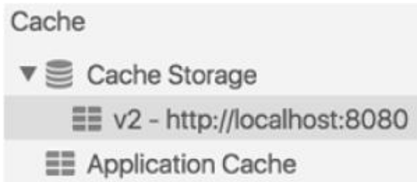
Figure 9.13. Your new v2 cache. If you click this, you'll be able to see the updated cache contents, particularly the global.css?v=1 entry.
