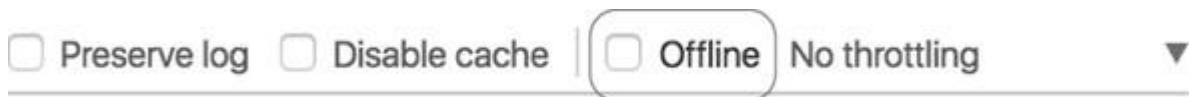
Figure 9.7. Selecting the Offline check box in Chrome's Network panel allows you to simulate what it's like to be offline without having to disable your network connection.
