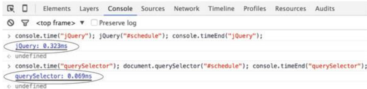
Figure 2.27. The results of two benchmarks you've run of jQuery's DOM selection versus that of the native document.querySelector method. Results are circled.
