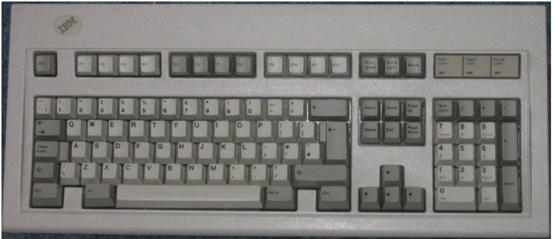
Figure 1-2. IBM modified the keyboard to include a separate cursor keypad along with a second cursor/numeric keypad
