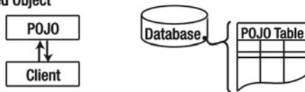
Figure 4-3. Detached objects exist in the database but are not maintained by Hibernate
