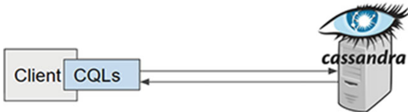
Figure 5-12. The native way to connect to a Cassandra server is via CQLs.
