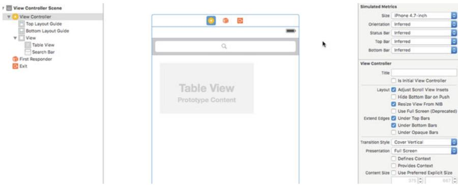
Figure 9-11. Adding the UITableView and UITableViewCell
