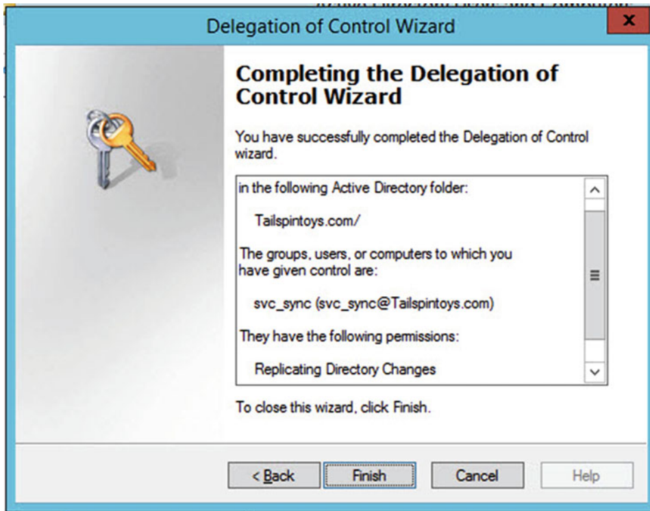
Figure 11-43. Scroll down to see only Replicating Directory Changes on the entire domain
