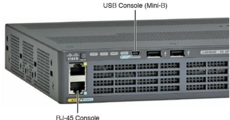
**Figure 6-4** A Part of a 2960-X Switch with Console Ports Shown
