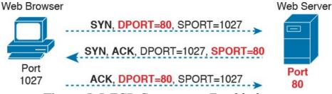
Figure 5-5 TCP Connection Establishment
