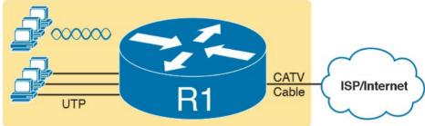
**Figure 17-5** *SOHO Network, Using Cable Internet and an Integrated Device*
