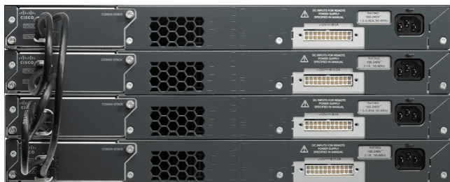
Figure 6-15 Photo of Four 2960X Switches Cabled on the Left with Stacking Cables
