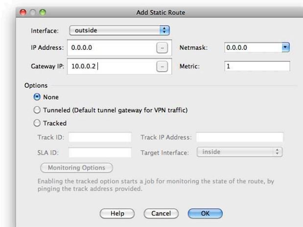
You can see from Figure 47 that a route is set to 0.0.0.0 0.0.0.0 that points to 10.0.0.2. The notation of 0.0.0.0 0.0.0.0 is the default catchall address, which can also be represented as 0 0.
