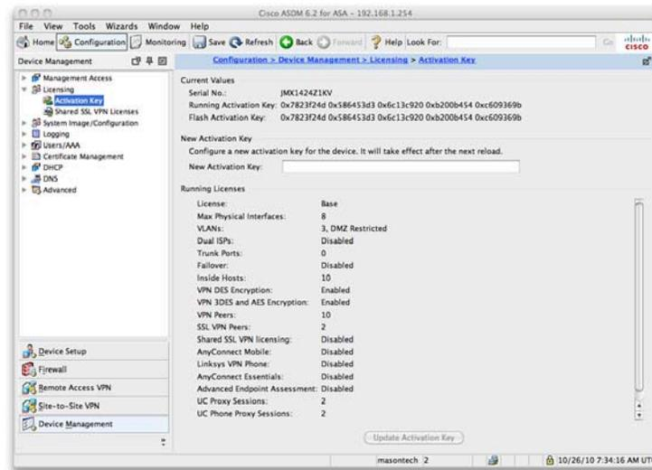
The current license and features can be seen from the Home screen and the Device Dashboard in ASDM as well as from this screen where the exact license details and what is enabled on the ASA you are connected to are shown.
