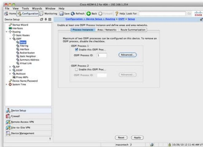
Clicking the Advanced tab brings up a set of configurable items for OSPF that can be seen in Figure 51:
