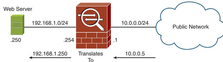
The web server has an internal IP address of 192.168.1.250/24. Hosts from the outside cannot access this server on this address because it is not routable via the outside interface (because a NAT translation is required).
