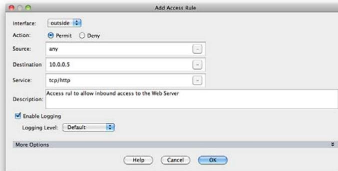
You can see from Figure 28 that you created a rule that permits TCP port 80/HTTP traffic from anywhere to access the outside interface and the address 10.0.0.5. This is the address you used for the static NAT translation for the web server.
