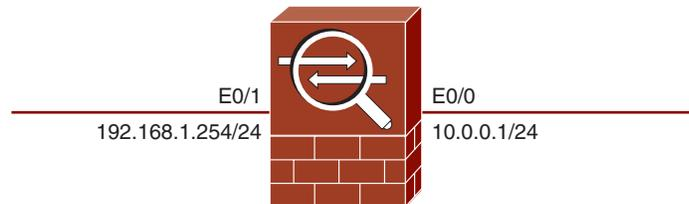
To assign an IP address to an interface, use the **ip address** command from interface configuration mode. The following example sets the IP address of 10.0.0.1/24 to Ethernet0/0:
