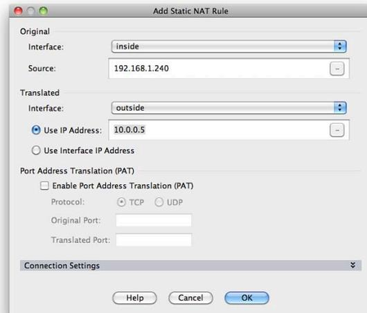
You can see in Figure 23 the entered original and translated addresses into the ASDM. This setting can translate 192.168.1.250 to 10.0.0.5 on the outside interface. When applying this setting, you then go back to the NAT Rules configuration screen shown in Figure 24. This screen lists all the configured NAT rules on the ASA, which in this case is only the single static NAT rule.
