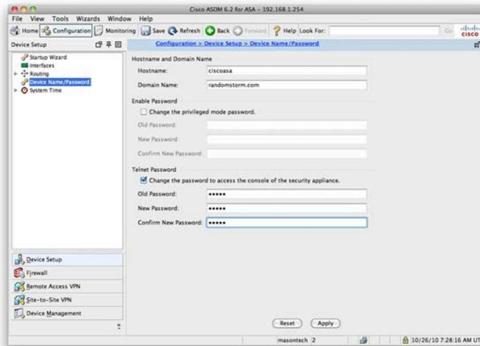
Telnet is now configured on the ASA, and users on the 192.168.1.0/24 network can telnet to the ASA.
