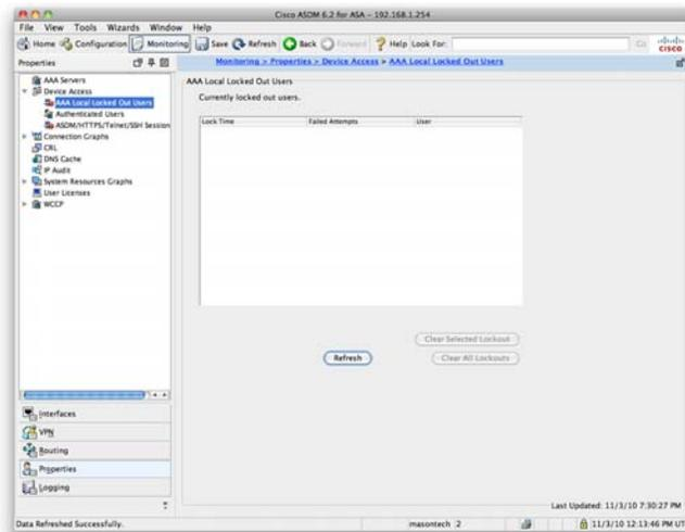
To reenable a locked account, select the locked-out account, and then click the **Clear Selected Lockout** button.
