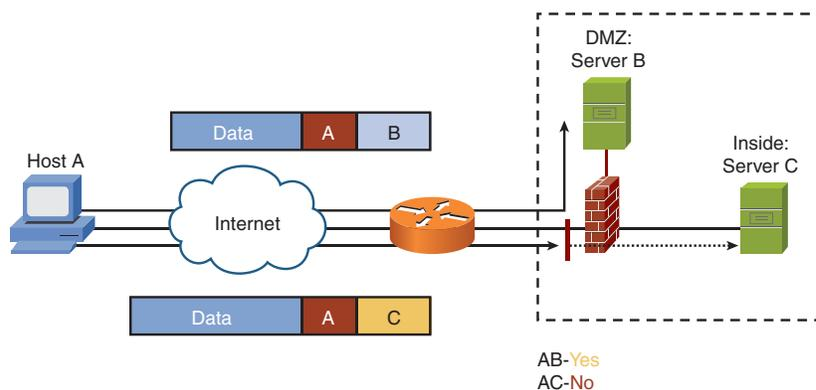
Most Cisco network devices perform some level of packet filtering implemented as ACLs.
