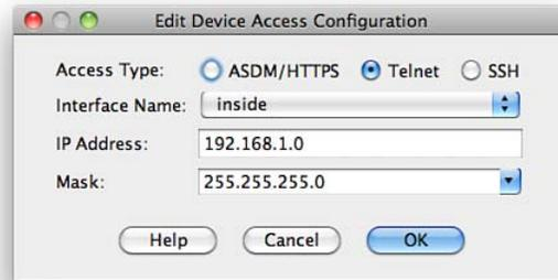
In Figure 14 you have enabled Telnet access on the inside interface for the network 192.168.1.0/24. You now have to enter a Telnet password into the ASA. Navigate to **Device Setup > Device Name/Password**. Click the check box to change the Telnet password. By default, the old password is set to cisco. Enter a new secure password, and then apply it. Figure 15 shows the Device Name/Password screen.
