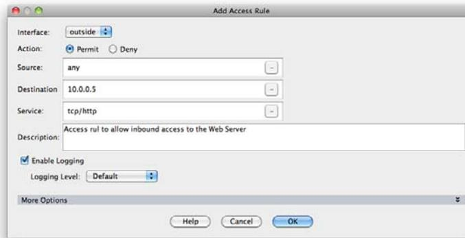
You can see from Figure 28 that you created a rule that permits TCP port 80/HTTP traffic from anywhere to access the outside interface and the address 10.0.0.5. This is the address you used for the static NAT translation for the web server.
