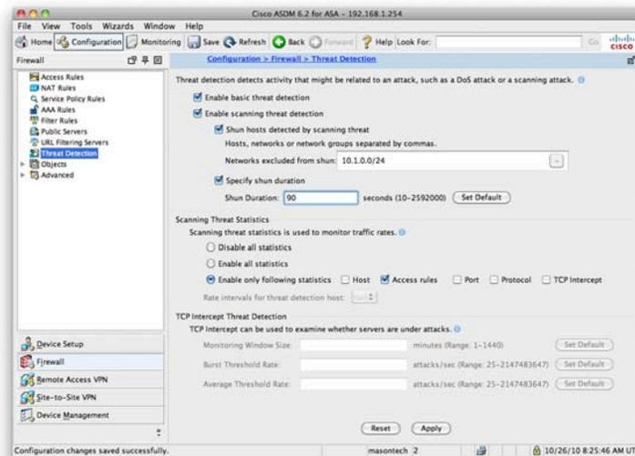
When a shun is activated, all current connections from the malicious host are dropped, and all future connections are blocked at the outside interface of the ASA. Shuns are dynamic in nature and are not stored as a part of the configuration. If the security appliance loses power or reloads, any active shuns are lost.
