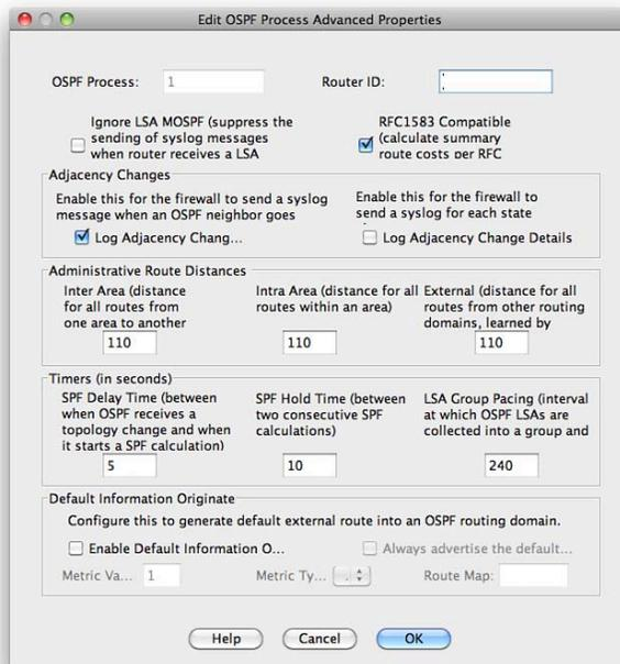
Click OK to leave these as they are and return back to the OSPF setup screen. The next step is to configure the OSPF areas and to place interfaces within an OSPF area. Use OSPF area 100, and place the inside network interface with the IP address of 192.168.1.254 in this area.
