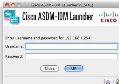
The authentication box requests a username and password. Because you have not configured any users on the system, you just need to enter the enable password into the Password field and leave the Username field blank. You are now presented with a connection to the ASDM (see Figure 9).
