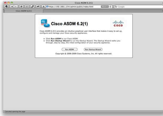
You can either run the ASDM or the Startup Wizard to take you through the initial setup of the ASA. Click the **Run ASDM** button to launch ASDM.
