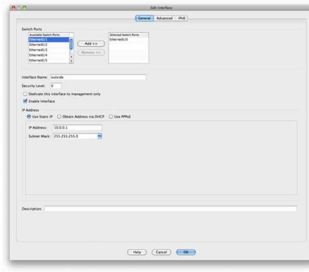
You can see in Figure 12 that Ethernet0/0 is assigned an IP address of 10.0.0.1/24. This interface is named outside and given a default security level of 0.
