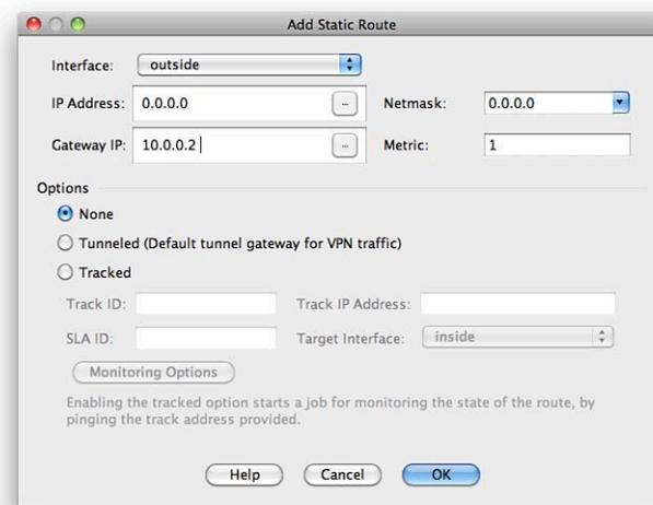
You can see from Figure 47 that a route is set to 0.0.0.0 0.0.0.0 that points to 10.0.0.2. The notation of 0.0.0.0 0.0.0.0 is the default catchall address, which can also be represented as 0 0.
