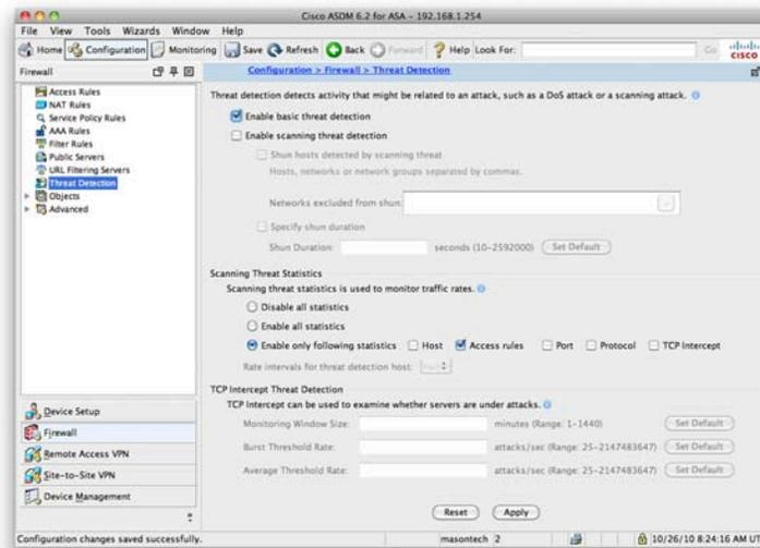
You can see from Figure 45 that basic threat detection is enabled on this ASA. To disable it, uncheck the check box.
