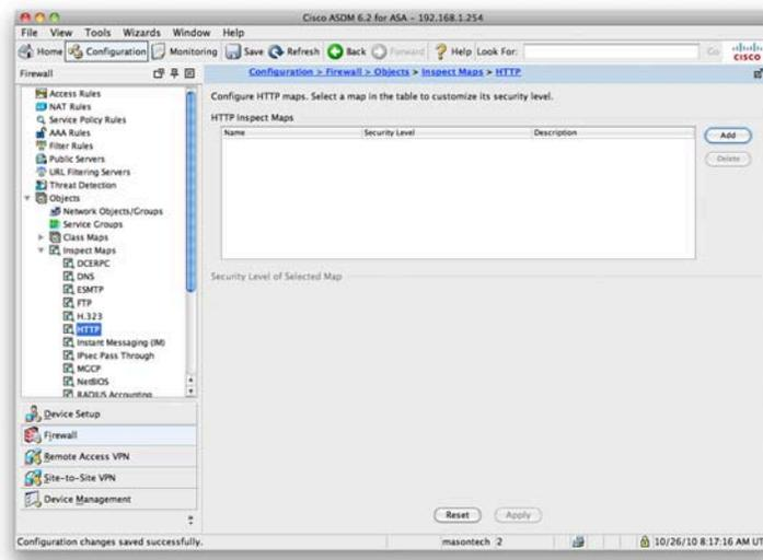
Clicking Add opens a new HTTP inspection policy map. You can either use one of the built in Security Levels of Low, Medium, or High, or you can click the Details button to configure individual inspection.
