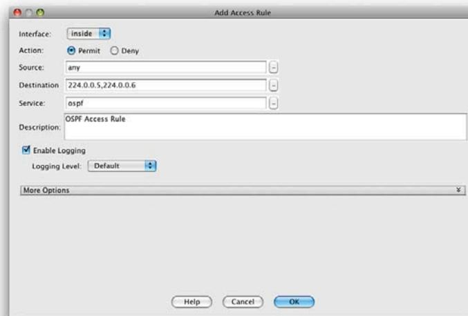
Then create a rule on the outside interface to enable OSPF to be allowed from the outside in. When this is applied, you are presented with the Access Rules screen, as shown in Figure 58.
