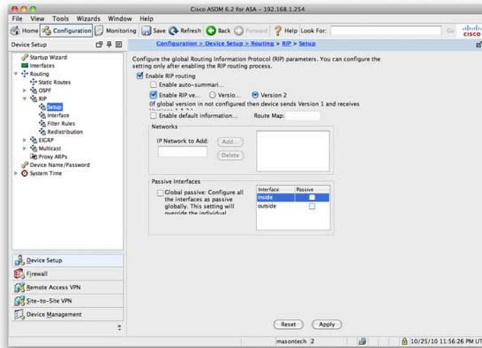
Figure 48 shows that you have enabled RIP; set it to use RIPv2. This setup configures RIPv2 on the ASA so that it fully participates in RIP routing, accepting routes from neighbors and transmitting routing updates to neighbors.
