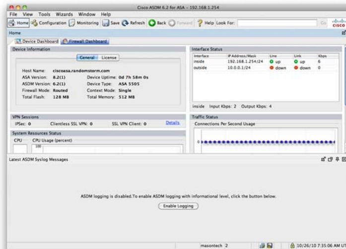
You can see from Figure 18 that ASDM logging is disabled. There is a button in the bottom half of the screen that can enable logging. Clicking this button enables logging on the ASA.
