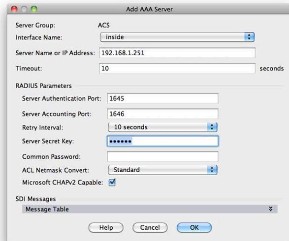
You now have the ACS AAA server group and the single server in that group. You can have multiple servers in a group for redundancy and for load balancing when the network is heavily used.
