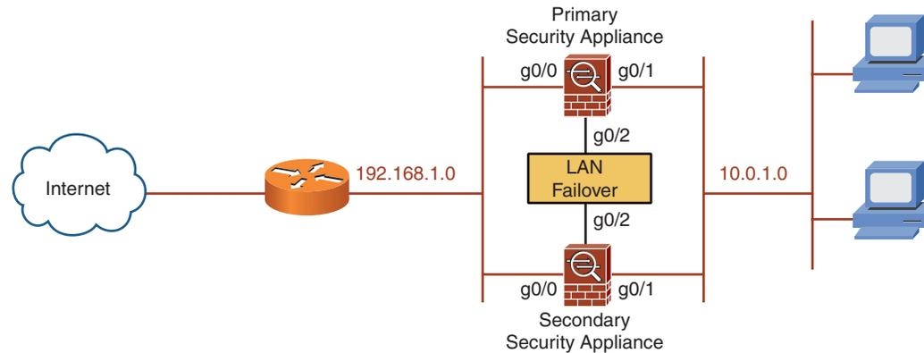
As shown in Figure 70, a LAN-based failover connection is required between the primary and secondary ASA. If you plan to use stateful failover, an interface on the ASA must be dedicated to this function, unless you configure stateful failover to share the same interface as the LAN-based failover connection.
