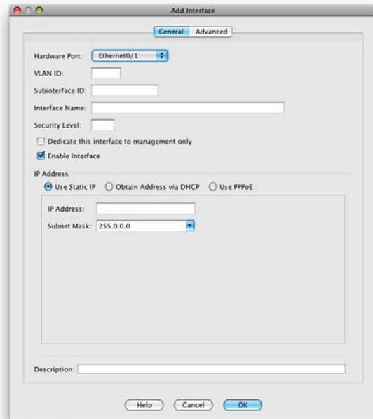
You can then select which interface this subinterface is to be bound to and set the options such as the VLAN ID and subinterface ID to configure the subinterface.
