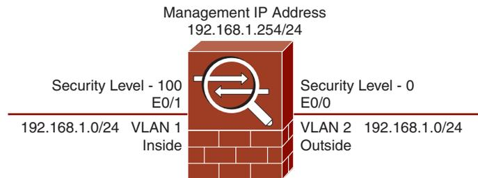
You now need to follow the steps outlined in Section 2 to set up the ASA so that you can access ASDM. In brief, enable and configure an interface, and enable the HTTP server on the ASA. When that is completed, you can connect to the ASDM using the 192.168.1.254 management address that you configured.
