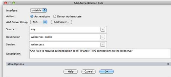
In this example, after the authentication rule is applied, users are prompted for a username and password when they start HTTP or HTTPS connections to 10.0.0.5 from the outside. The AAA server verifies whether the username and password are correct. If they are correct, the security appliance cut-through proxy permits further traffic between the initiating host and the target host.
