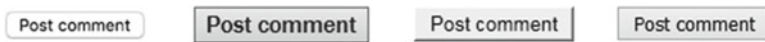
Figure 9-15. Unstyled button elements from Chrome on OS X, IE10 on Windows 7, Firefox on Windows 7, and Microsoft Edge on Windows 10
