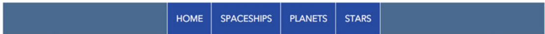
Figure 6-27. Centering flex items with justify-content: center. Extra space is placed on the outer sides of the edge items
