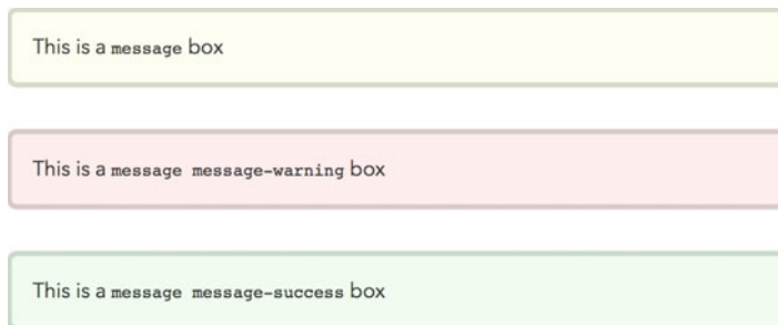
Figure 12-11. A smart structure allows us to quickly create other flavors of message boxes
