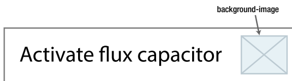
Figure 5-8. A piece of text with an icon as a background image at the right edge
