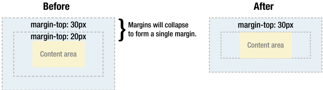
Figure 3-8. Example of an element's top margin collapsing with the top margin of its parent element
