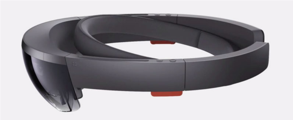
Figure 13-4. The visor is not aligned with the head band
