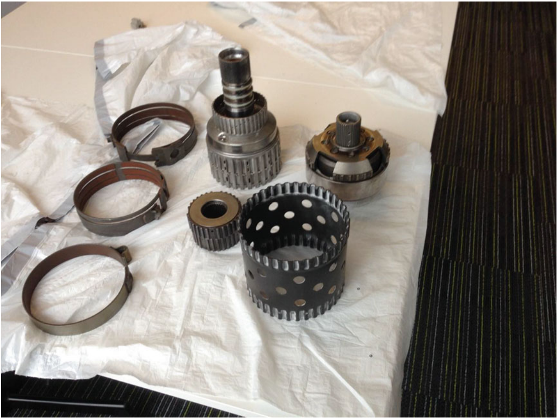
Figure 16-5. Automatic transmission in pieces
