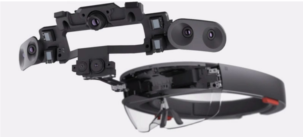
Figure 13-5. Cameras and light sensor
