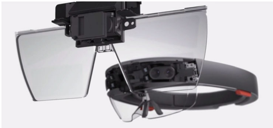
Figure 13-6. Lenses, light engines, and IMU
