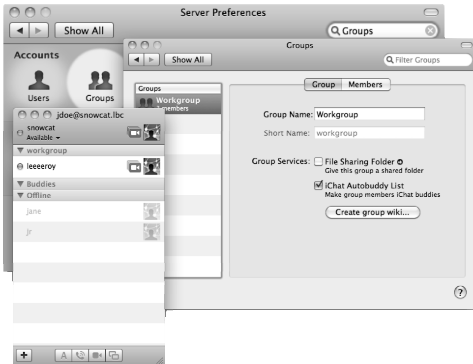
Figure 5-31. Configuring iChat Autobuddy Lists in Server Preferences (back) and the resulting iChat buddy list (front)
