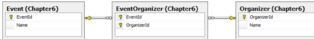
Figure 6-2. A database diagram showing the EventOrganizer link table holding the foreign keys to the related Event and Organizer tables
