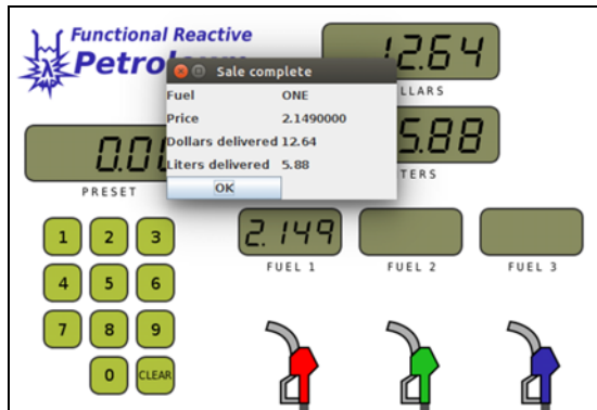
Figure 4.3 When you hang up the nozzle, the sale details are sent to the point-of-sale system.
