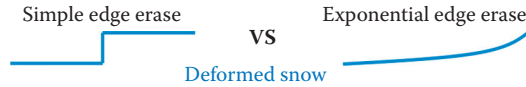
Figure 1.13. Exponential edge erase provides a much smoother finish to the trails over a more simple approach.
