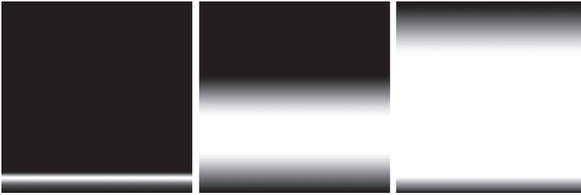
Figure 4.10. The gradients produced by three density height functions to represent stratus (left), cumulus (center), and cumulonimbus (right) clouds.
