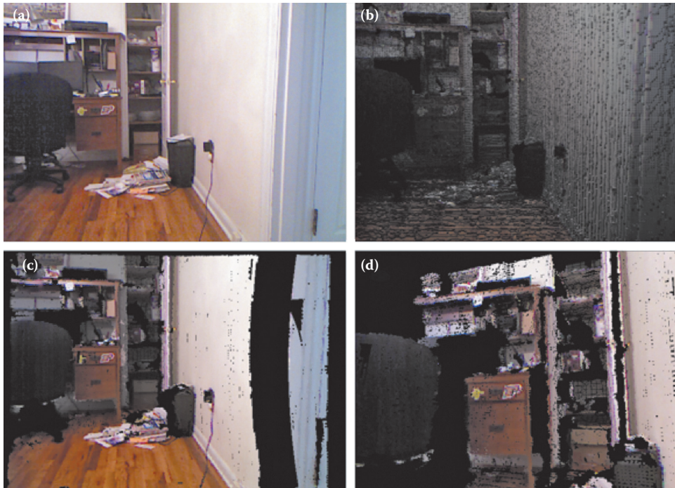
Figure 1.5. Octree scene constructed from a live Kinect camera stream using CUDA. (a) The original raw camera image. (b) Voxel extraction and instanced rendering of an SVO map. (c) Voxel cone tracing of an SVO map. (d) Voxel cone tracing from a virtual camera view that does not match the physical view.
