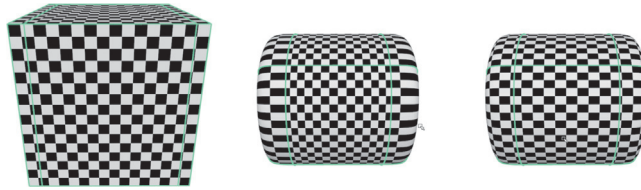
Figure 2.16. From left to right: A textured cube control mesh with beveled caps, the surface with linearly interpolated texture coordinates, and the surface with smoothed texture coordinates.
