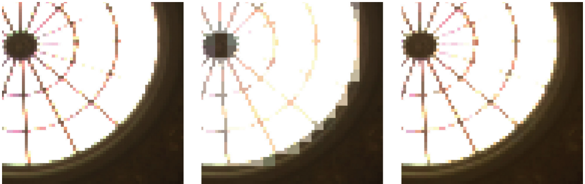
Figure 2.1. Endpoint algorithm: reference (left), compressed using bounding box inset (center), and compressed using bounding box refine (right).
