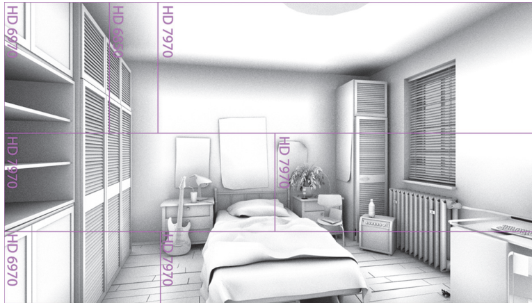
Figure 4.5. Bedroom scene rendered using three machines connected via 10-Gb Ethernet. The frame is split horizontally to distribute the work for machines. In each machine, the frame is split vertically on GPUs. We used 4 \times AMD Radeon HD 7970, 2 \times AMD Radeon HD 6970, and 1 \times AMD Radeon HD 6850.
