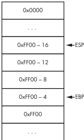
Figure 4-8: Example stack with stack frame set up (read from bottom to top)
