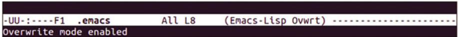
FIGURE 11-9. Mode line showing the major mode as well as one minor mode.
