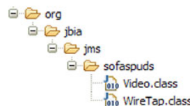
Figure 8.10 The example MDB JAR file contains two classes: the Video class (the object passed in the messages) and the WireTap class (implements the message-driven EJB).
