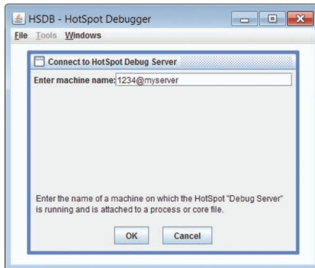
Figure 4.7 Connect to HotSpot Debug Server
