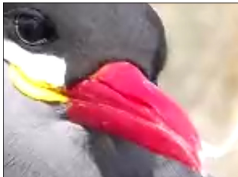
FIGURE 9-13: MPEG-4 part 10 compressed I frame. Notice how there are few artefacts (the slight blurriness is because it's zoomed in to show detail).
