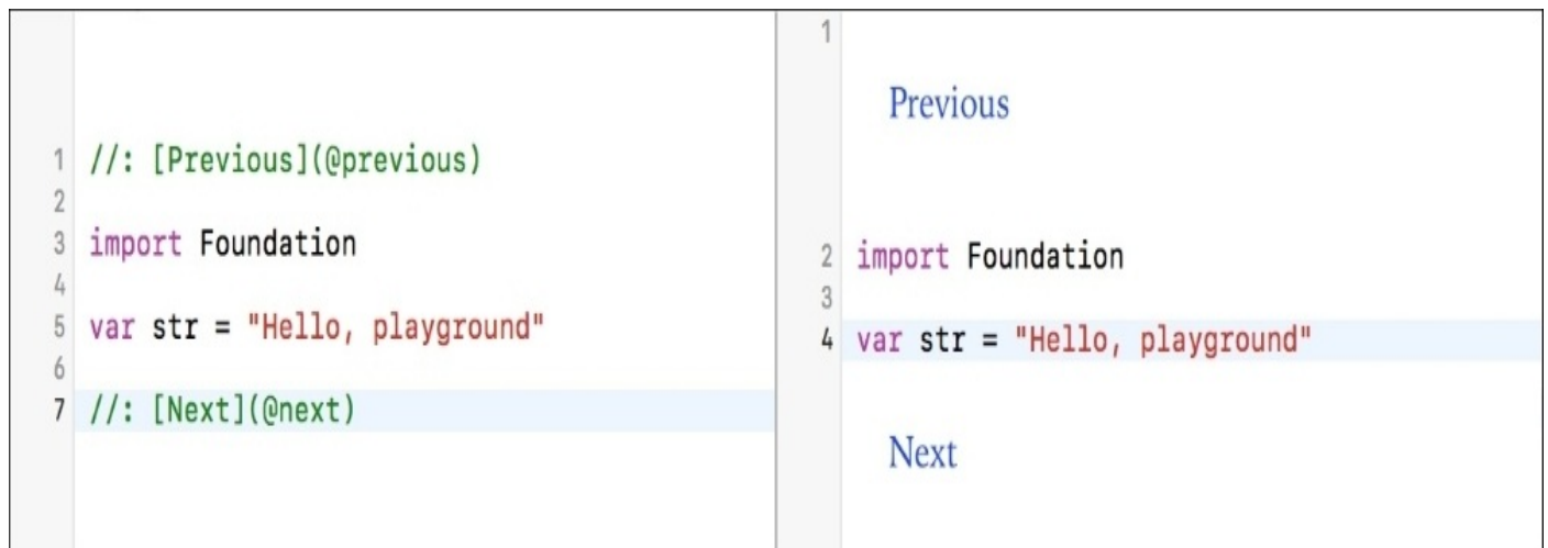
Figure 3.8: Special code comments (shown on the left) create previous and next buttons (shown on the right)
