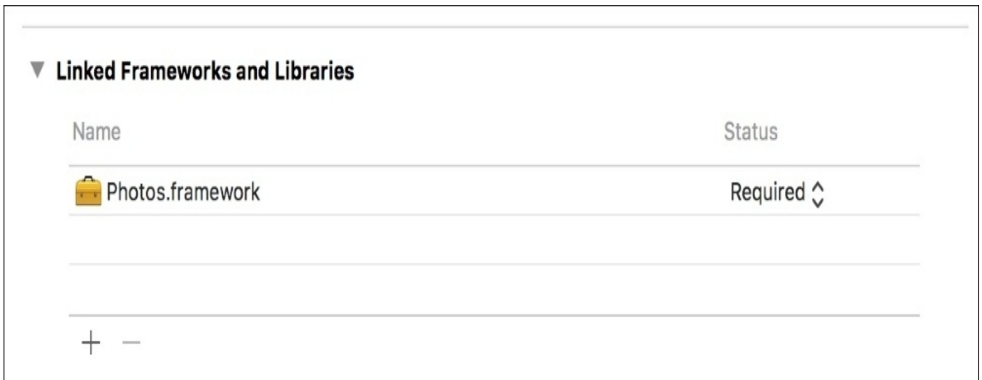
Figure 8.2: Choosing Photos.framework from the drop-down list adds it to our Linked Frameworks
