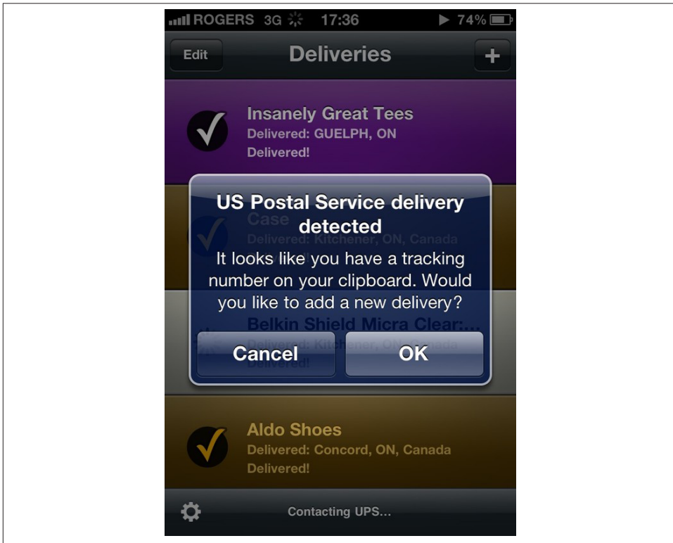
Figure 2-19. The deliveries app checks if there is a tracking number in the clipboard on launch, and if so, a system trigger launches this microinteraction. It's also smart enough to indicate from which courier the number is from. (Courtesy Patrick Patience and Little Big Details.)
