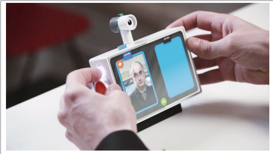
Figure 6-5. A still from a prototype movie. The physical pause button on the left “shoots” a pause indicator out onto the screen. (Courtesy BERG London)
