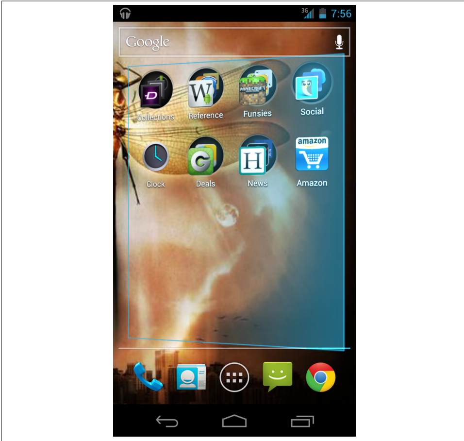
Figure 4-23. In Android (Ice Cream Sandwich versions), the screen skews if you try to scroll past where there are items. (Courtesy Tony Mouch and Little Big Details.)
