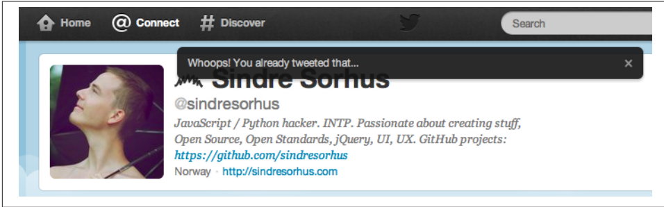
Figure 3-33. Twitter won't let you tweet the same message twice, mostly to protect its service from abuse. Detecting a duplicate before the user presses Send would be better, although more system-resource intense. (Courtesy Sindre Sorhus and Little Big Details.)
