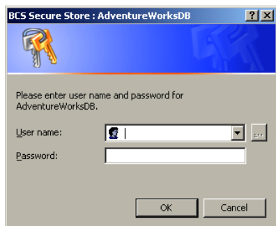
FIGURE 4-14 When you use impersonation authentication methods, you are prompted for credentials that SharePoint Designer can use to directly connect to the data source.
